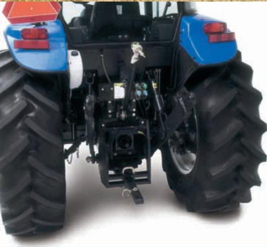
*Left: Flexible link ends and telescopic stabilizers are standard equipment for easier three-point implement hookup.*
