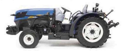
low clearance applications. The height of cab models has been reduced by 5.2 inches versus the previous TNV-A Series, with the relocation of the air conditioner condenser, providing a minimum height of 84.6 inches (depending on tire size). Open station tractors feature a mid-mount rollbar that folds down, permitting a minimal overall height of 50.8 inches.
