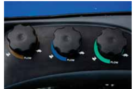
Flow control for all three cab-end remotes is provided inside the cab for your convenience.
