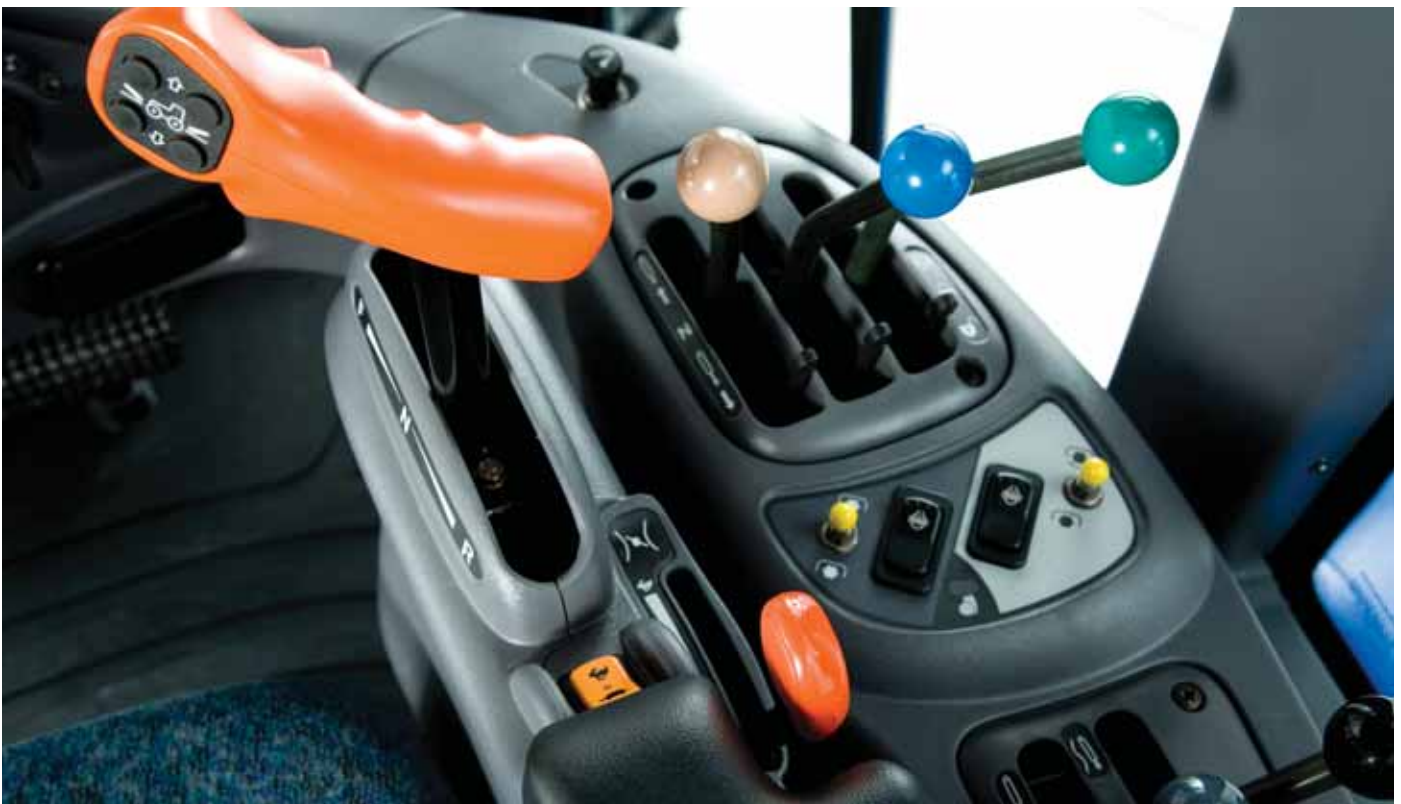
Flow control for all three cab-end remotes is provided inside the cab for your convenience.
