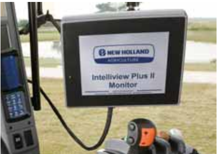
The New Holland IntelliView Plus II touchscreen color monitor provides complete interface with the IntelliSteer system for fingertip control of operation, data storage and calibration.
