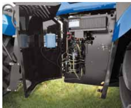
Reach batteries, washer fluid and axle lube filter through this handy right-hand service door. Steps on the door let you use a service-access window to reach the electrical components in the cab and easily route monitor cables.
