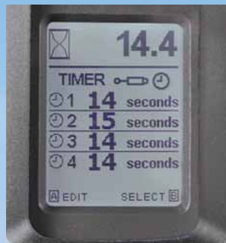
Performance instrumentation provides individual remote timers and a visual read-out of flow control settings.
