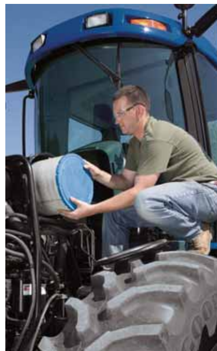
The engine air filter is located under the hood for more efficient air flow, longer filter life and easy access.
