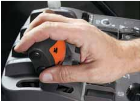
Change speeds with the touch of your thumb with the 16-speed powershift.
