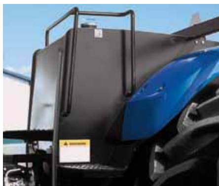
A 300-gallon fuel tank is integral with the rear frame to keep refueling to a minimum and your productivity to a maximum (200 gallon tank on the T9020).
