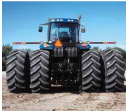
Here's a closer look at the large-diameter 4WD wheel tractor bar axle—one with the strength and durability to match the high-horsepower and heavy-load capability of T9030HD, T9040HD, T9050HD and T9060HD tractors, as well as all scraper models.
