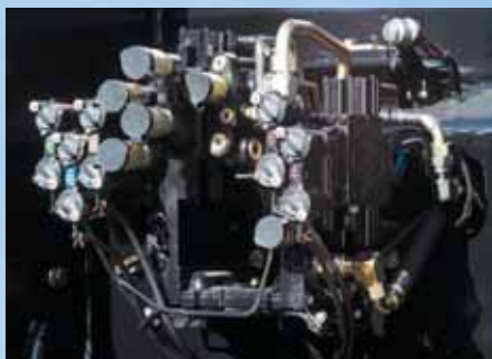
Up to nine remote valves and MegaFlow™ can be built into any T9000 model. Seven remote valves and power beyond are pictured.
