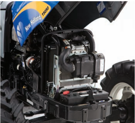
T5000 Series engines are turbocharged and intercooled for increased fuel efficiency.
