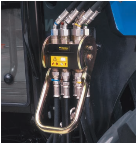
The optional Fast-Snap feature allows you to disconnect all four loader valves with one lever.
