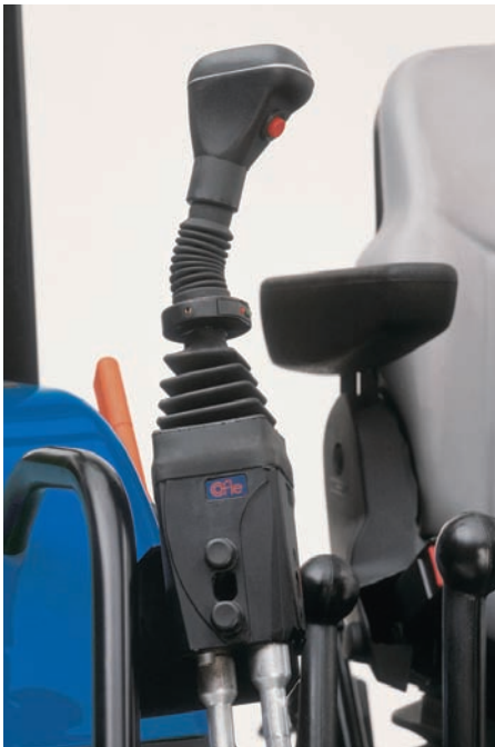
A convenient four-way joystick control is ideal for loader control.
