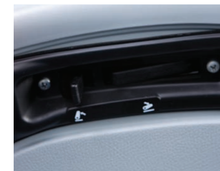
The Lift-O-Matic™ button allows you to instantly raise or lower the three-point hitch—a handy feature not usually offered on other tractors of this size.
