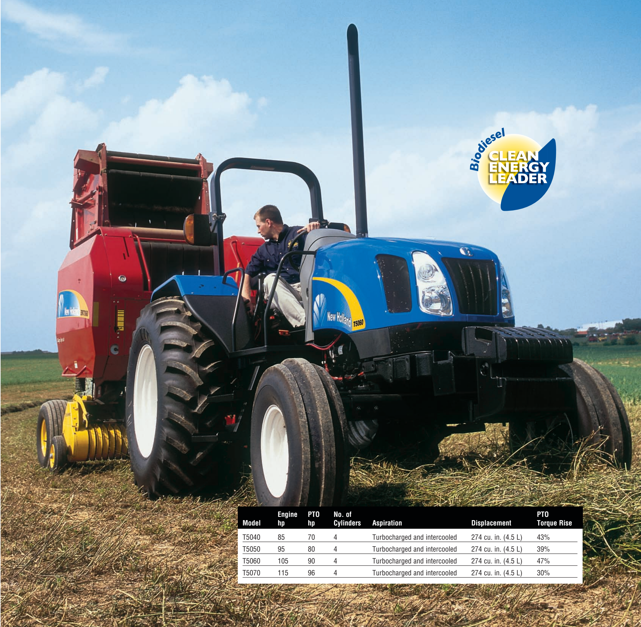
T5000 Series engines are turbocharged and intercooled for increased fuel efficiency.
