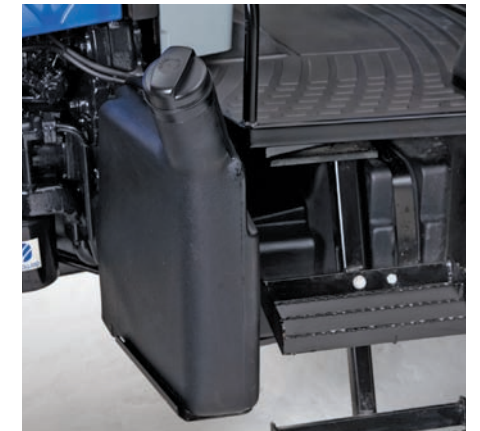
A 33.5-gallon fuel tank on all models keeps fuel-fills to a minimum. The low fill point location and wide filler neck make refueling easy.
