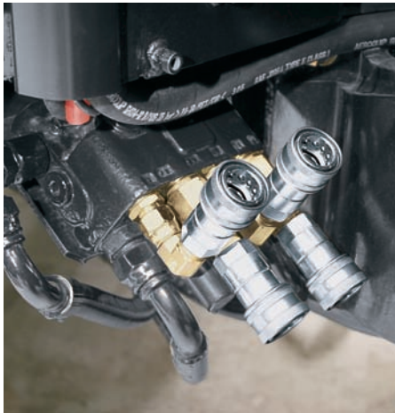
Mid-mount hydraulic valves make it easy to attach and remove New Holland loaders.
