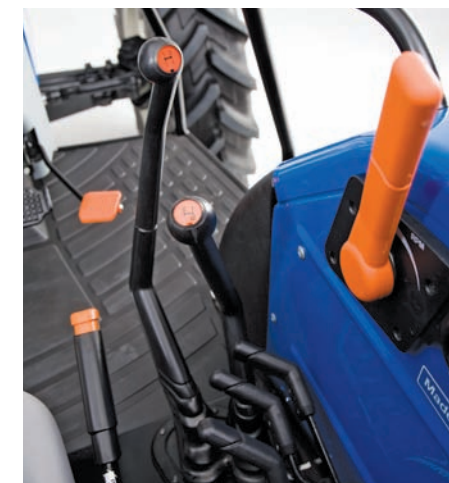
Speed and range levers for either transmission are located conveniently to your right and are easy to reach.
