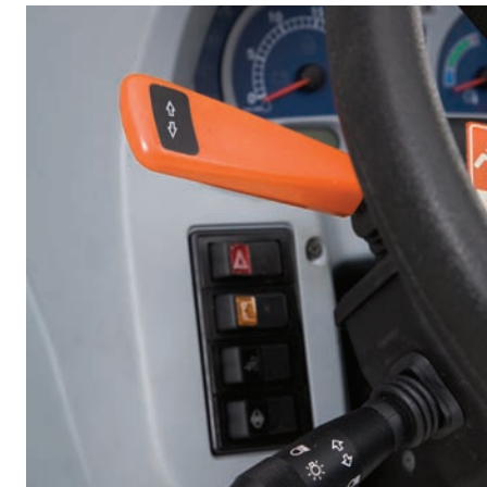
The power shuttle lever allows you to shuttle from forward to reverse without clutching and without removing your hands from the wheel. The power shuttle is standard on Deluxe T5000 models and optional on T5000 Standard models.
