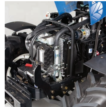
Easy access to filters, radiator, coolers and battery saves you valuable time.
