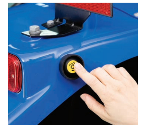
Convenient fender-mounted PTO switches (T5000 Deluxe models) start and stop the PTO with one touch, and make it easy to attach implements from the ground.
