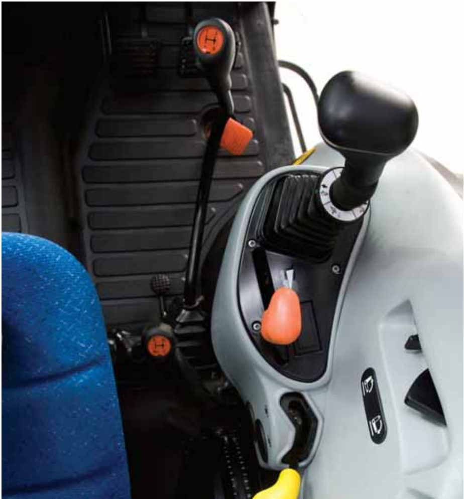
Speed and range levers are located within easy reach of your right hand.
