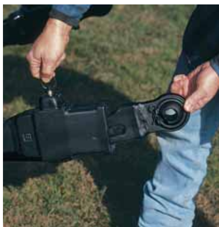
Heavy-duty, telescoping stabilizers and flexible link ends simplify implement hook-up and allow for quicker implement swapping.
