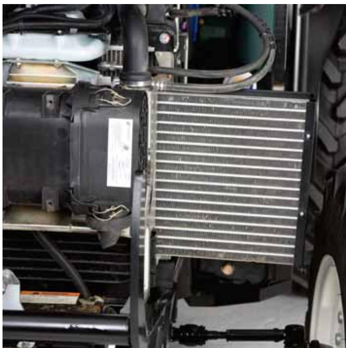
The hydraulic cooler slides out to the side for easy cleaning.
