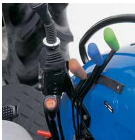
Rear remote lever controls are located to the right of the seat. Their handles are color-coded to match the caps on the valve couplers at the rear of the tractor, so you're always sure you're using the correct lever.
