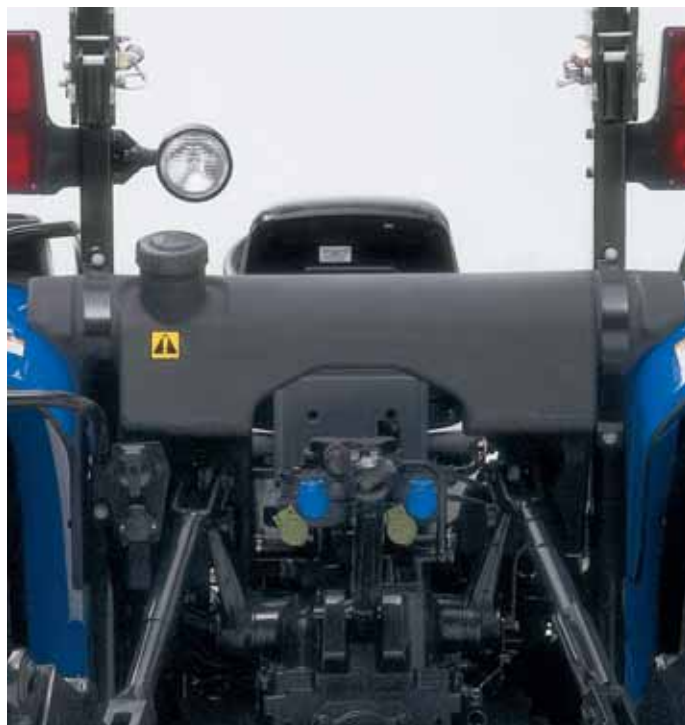
The fuel tank is easy to reach from the ground. Fuel tank capacity ranges from 19.8 to 23.2 gallons, depending on model, and keeps refills to a minimum.
