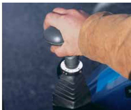
A simple, four-way joystick control makes operating the loader easy.
