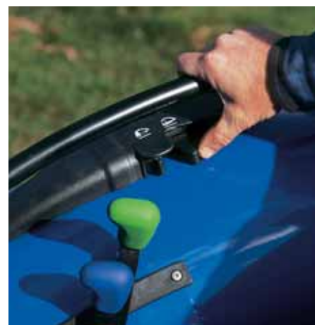
Here's a convenience not found on competitive-brand tractors: raise or lower implements with the simple push of a button
