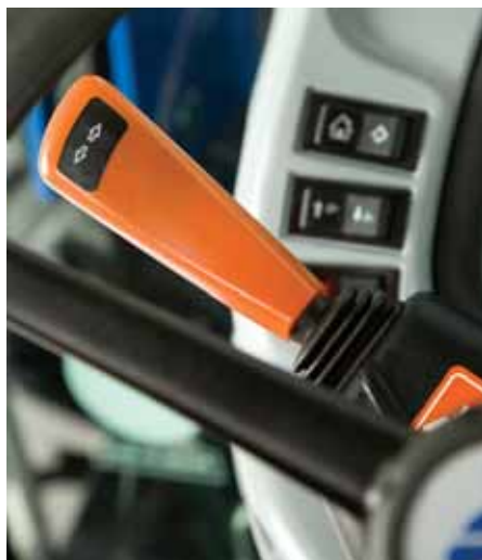
This power shuttle lever, available on all models, allows you to keep your hands on the wheel and shift from forward to reverse with your fingertips. It's the ideal choice for loader work.
