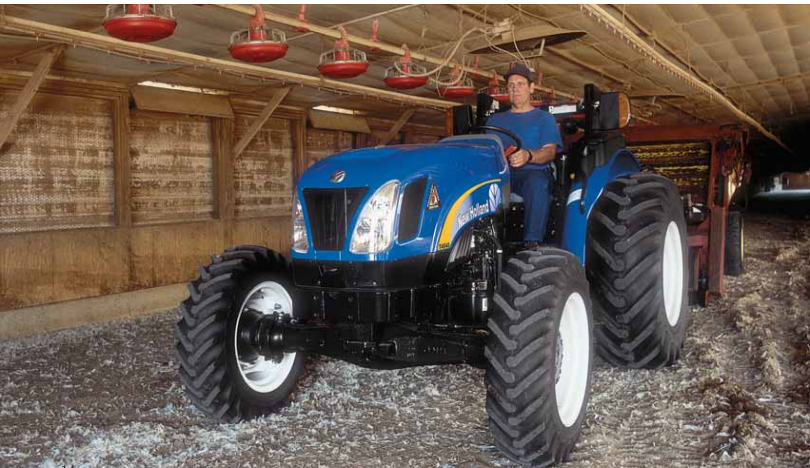
This power shuttle lever, available on all models, allows you to keep your hands on the wheel and shift from forward to reverse with your fingertips. It's the ideal choice for loader work.
