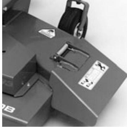
Clippings are distributed evenly through the right-side discharge with spring-loaded shield.
