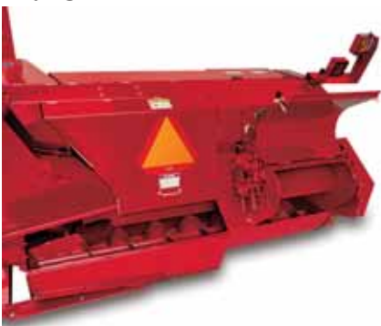
A seven-foot-long, 11 \frac{1}{8} -inch-diameter cross-flow auger moves silage from the crop processor to the blower fan.
