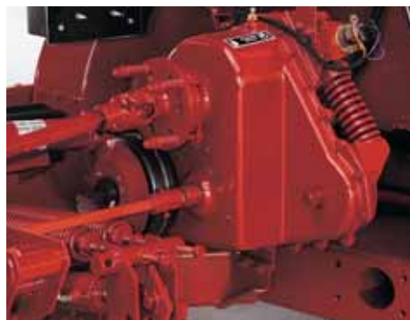
A special gearbox permits reversing the feedrolls and header drive to clear heavy slugs in case of overload. An electric clutch provides immediate response and positive control of the gearbox.
