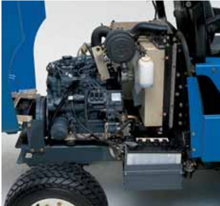
The engine is fully enclosed with a one-piece hood that flips up to provide fast, easy access to all routine maintenance areas.
