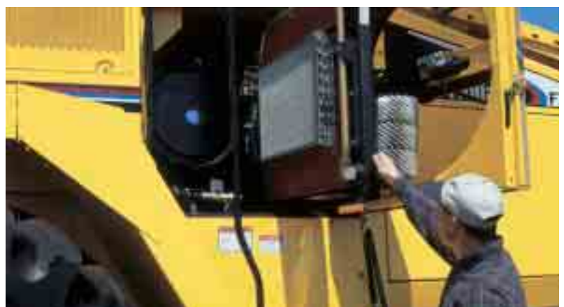
The oil cooler, air conditioning condenser, air-to-air intercooler and engine radiator slide out on the left side of the machine for easy access. Doors open wide for easy cleaning of the two rotary dust screens.
