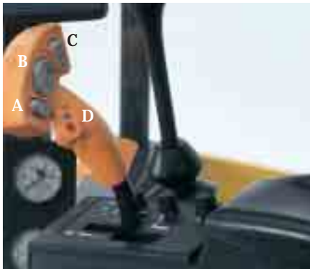
This lever allows you to control multiple functions with the touch of your thumb, including (A) feedroll and header drive, (B) spout deflector; rotation and dual-angle flipper, (C) header height, and (D) quick stop button. On the back side of the multifunction lever are controls for autopilot and automatic header height.
