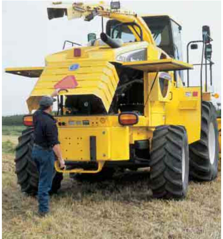
Engine guards open from the sides and rear, for plenty of light and open access for servicing and maintenance.
