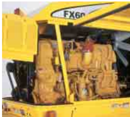
Six-cylinder, turbocharged and intercooled engines deliver a 25% torque rise between 1800 and 2100 rpm.
