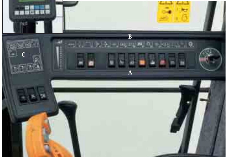
This electronic control panel to your right includes operating switches (A), including the metal detector, work lights, power reverser and four-wheel drive, as well as a row of indicator lights (B) that keep you informed at a glance. Controls for the Accucut™ sharpening system (C) are neatly grouped on one control panel.
