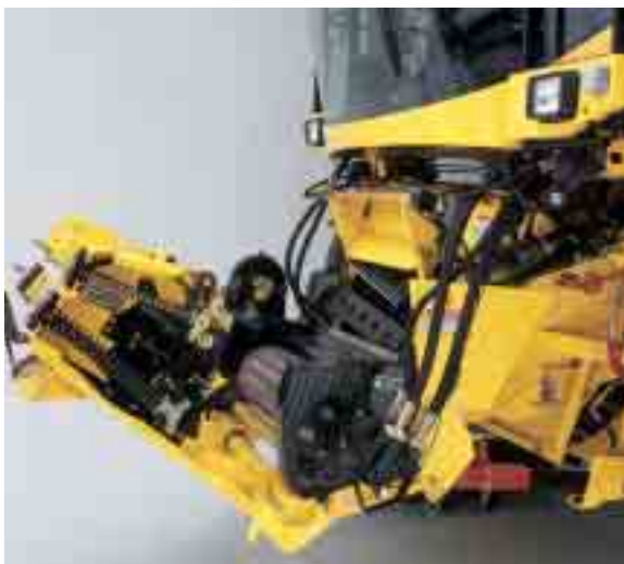
The oil cooler, air conditioning condenser, air-to-air intercooler and engine radiator slide out on the left side of the machine for easy access. Doors open wide for easy cleaning of the two rotary dust screens.
