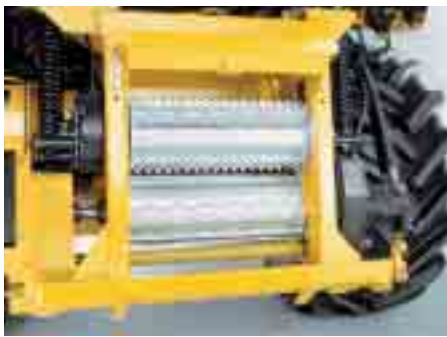
This wide feedroll opening provides maximum crop intake. The new HydroLoc™ hydrostatic feedroll drive allows you to change length-of-cut on-the-go.
