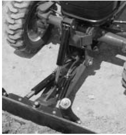
Blade lift is controlled hydraulically with this cylinder on the model 702C.
