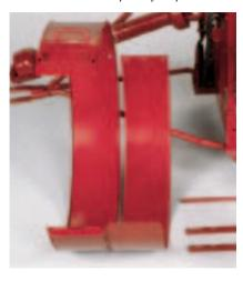
Replaceable fan wrapper liners are made of abrasive-resistant steel to increase blower life.
