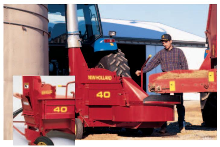
A convenient access door makes it easy to check fan-blade-to-band clearance and to replace fan paddles.
