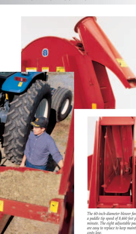
The "F62B" has a hinged blower outlet assembly so it's easy to inspect and maintain the fan paddles.
