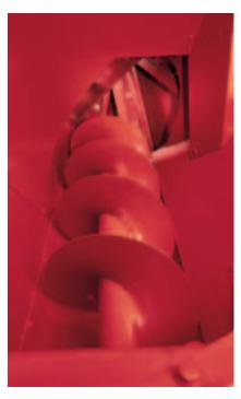
The new Model F62B forage blower has a direct-feeding auger positioned at a 30-degree angle to quickly move material into the high-capacity hopper.
