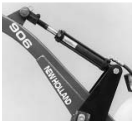
An optional down pressure kit for the heavy-duty model provides extra digging force for drilling in hard and heavy soil.
