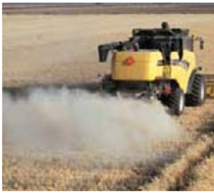
New Holland's optional straw chopper delivers superior chop quality. You adjust the right-hand and left-hand spread with a single lever, or add the optional in-cab adjustment.
