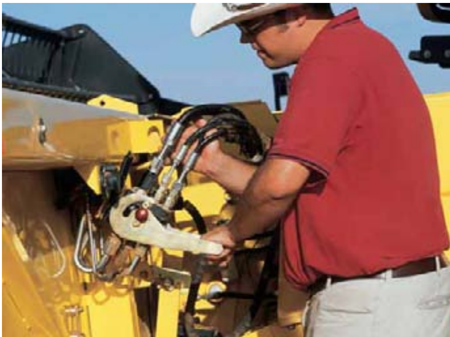
An easy, one-lever latching system on the left side of the feeder house operates both left and right latches simultaneously. A hydraulic multi-coupler engages all hydraulic lines with one over-center latch. It eliminates the need to hook up each head hydraulic circuit one at a time. It's a system that's quick, convenient and far less messy.
