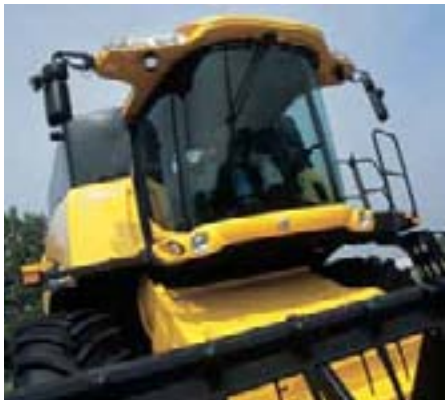
Up to six stadium worklights frame the top of the windshield, with additional lights under the windshield, as well as two side "row-finder" lights. Four rearview mirrors are standard and two more are optional. You can position the two larger mirrors electrically from the cab.
