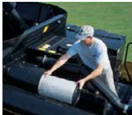
A large rear service deck provides easy access to all major engine service points as well as the grain tank.
