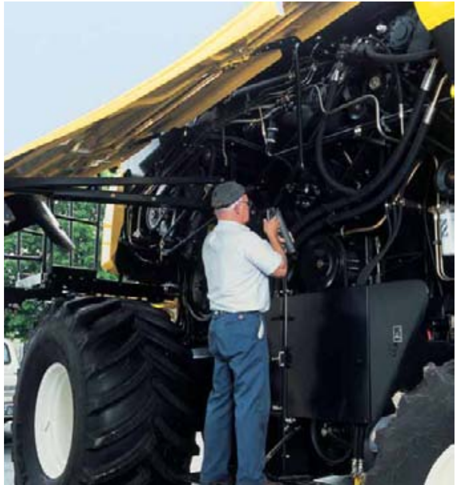
“Gull-wing” side shields provide complete service access.
