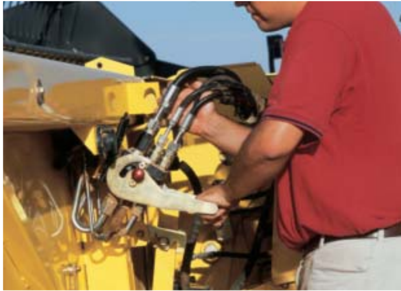
This hydraulic multi-coupler engages all hydraulic lines with one, over-center latch. It eliminates the need to hook up each header hydraulic circuit one at a time. It's a system that's quick, convenient and far less messy.
