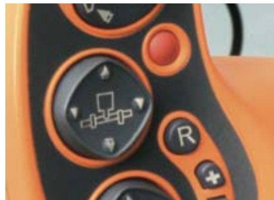
Terrain Tracer™ can be controlled manually with a switch on the hydrostatic lever.
