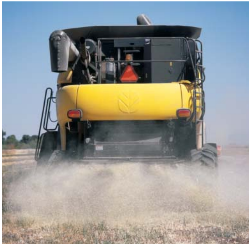
New Holland's straw chopper delivers superior chop quality. You adjust the right-hand and left-hand spread with a single lever, or add the optional in-cab adjustment.
