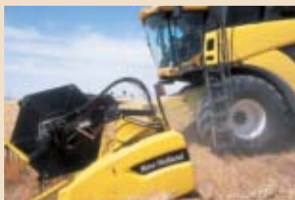
The long feeder and huge, curved windshield provide outstanding visibility to the cutterbar and after cut to take the strain out of operation.
