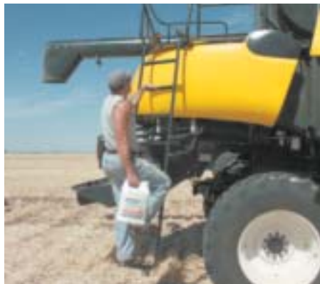
Rear service deck ladder folds down, making it easy to refuel or carry containers of fluid to the rear deck.
