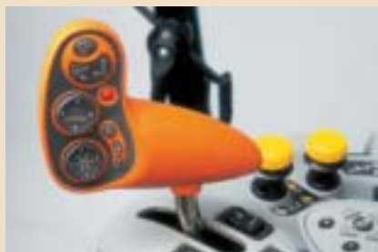
This adjustable-position, multi-function handle gives you inline control of the combine's hydrostatic drive, as well as controls for head height, head-tilt, reel speed, reel position, unloading auger engagement and swing.
