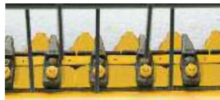
Hydraulic-driven, dual, counter-stroking sickles are belt-timed for a swift 1828-spm knife speed for fast, clean cutting.
