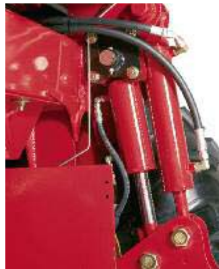
Adjustable cut height cylinders on each lift arm make it easy to return to the pre-set cutting height after each pass.
