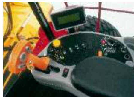
The floating operator console moves along with the seat to keep you comfortably in control at all times.
