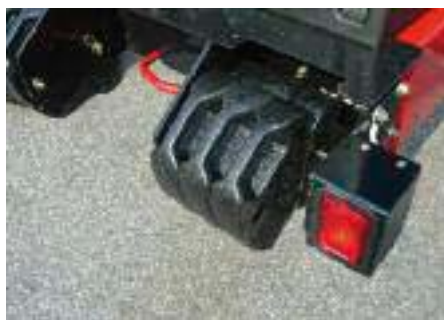
Optional rear weight bracket and weights may be installed on any H8000 model to balance heavy or wide heads.
