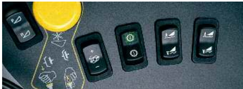
Dual switches in the H8060 and H8080 cab allow you to control the flotation of the left and right side of the header independently.
