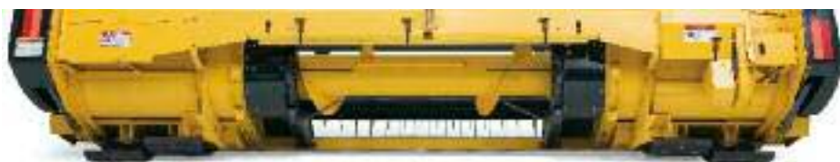
The wide opening in the header floor behind the cutterbar allows for gentle crop collection and windrow formation with the assistance of windrow forming rods.
