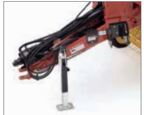
A heavy-duty hitch jack provides easy tractor hookup with jacking heights of up to 22 inches. Once the baler is hitched to the tractor, you can easily relocate the jack up and out of the way to avoid interference with the tractor's three-point hitch arms, tractor tires and crop windrows.
