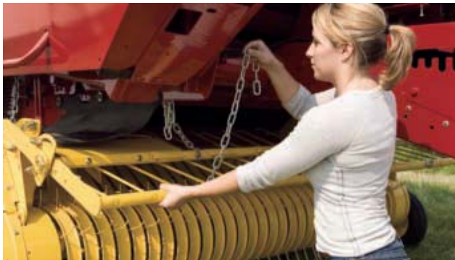
Adjustable windguards help control flow of crop from the pickup into the bale chamber.
