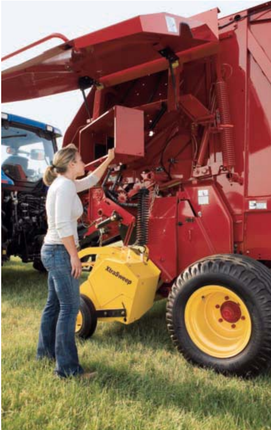
Gull-wing doors on both sides of the baler make daily maintenance a simple process.
