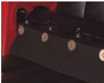
Three rolls have scrapers to remove crop that can build up on the rolls.
