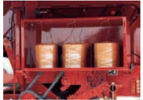
Side-load twine storage boxes hold six balls of twine on the BR7060, BR7070, BR7080 and BR7090 Auto-Wrap™ balers. An additional five or six balls of twine (depending on the model) can be stored in an optional front storage box on Auto-Wrap balers. All twine-net balers hold six balls of twine and two rolls of net.
