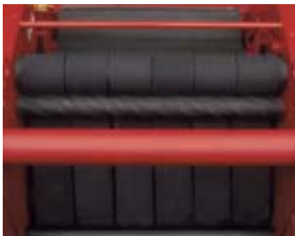
A rubber back wrap roll eliminates crop build-up on the back of the belts.
