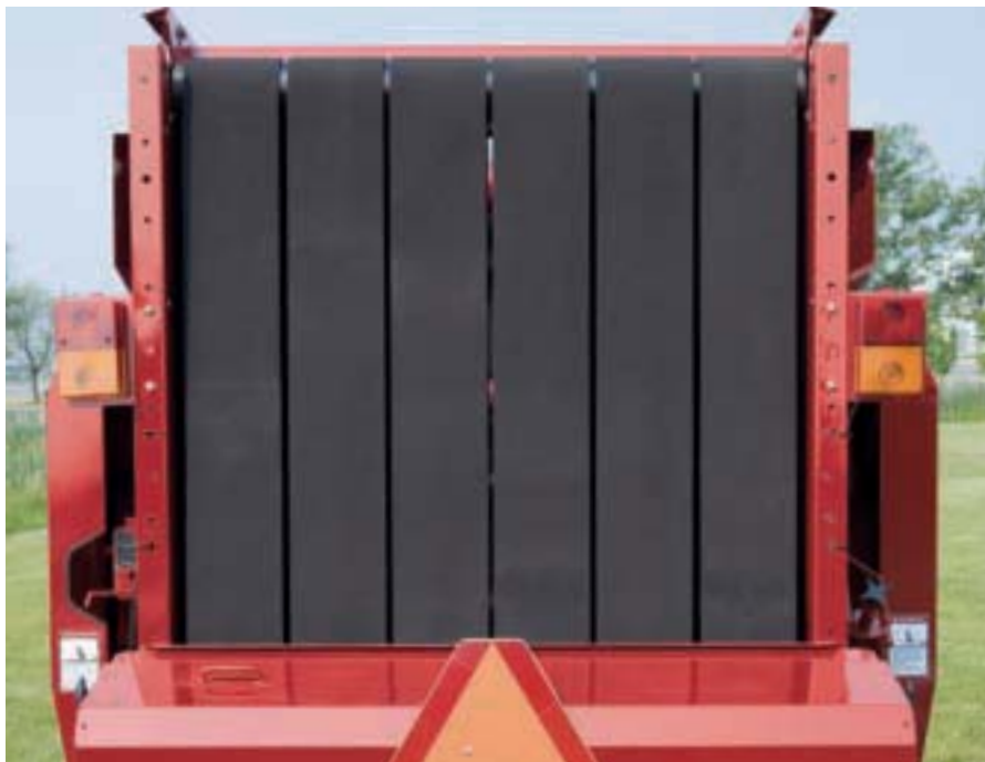
Endless belts eliminate the splice and the fastener maintenance required with laced belts. Even better, they're backed by an exclusive Bonded Protection Plan. If a belt fails due to defects in material or workmanship within the first three years or 15,000 bales, New Holland will replace it free.
