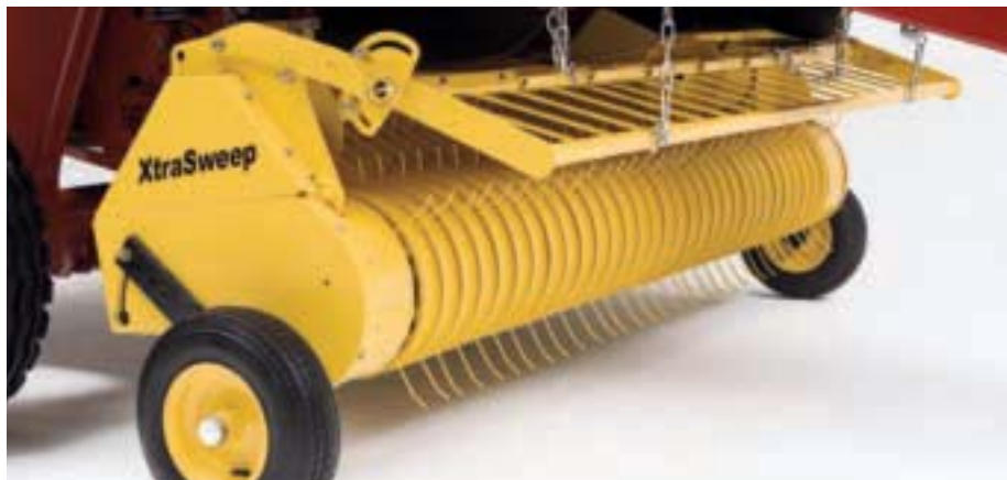
Both XtraSweep™ pickups use the same full-width, dual-pivoting windguard for total crop control into the bale chamber and two flotation gauge wheels to follow contours in the field.
