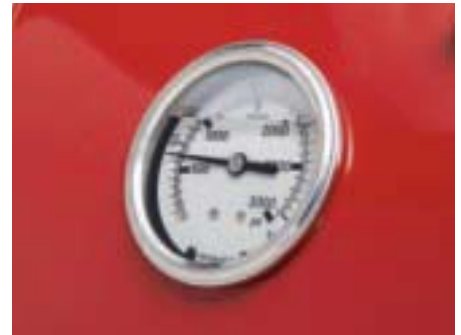
The calibrated density pressure gauge indicates bale density pressure in psi.
