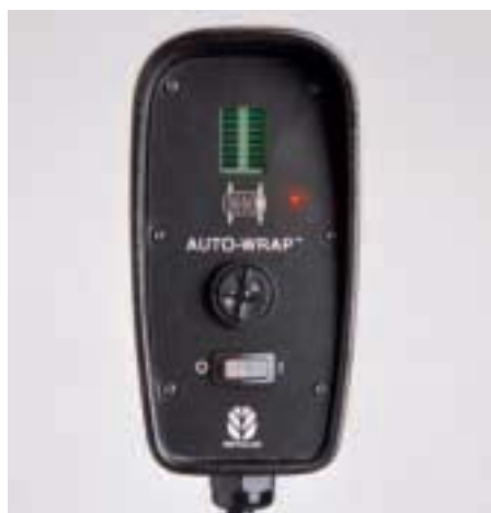
The Auto-Wrap™ bale shape monitor mounts inside the tractor cab. It helps operators make dense, uniform bales by showing which side of the baler needs more crop. A bale size indicator located on the right/front of Auto-Wrap balers monitors bale diameter.
