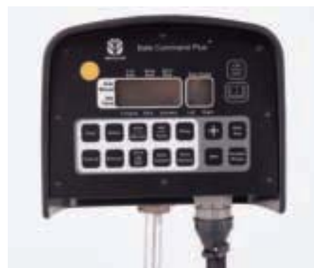
With the Bale Command Plus™ system, all baler functions plus tying or wrapping are closely monitored right from your tractor seat.
