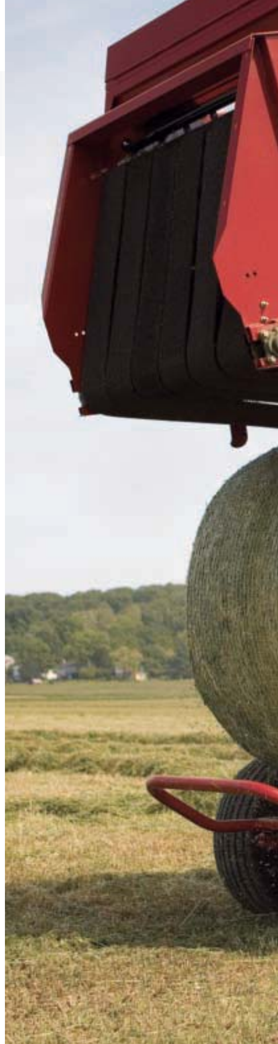
A rubber back wrap roll eliminates crop build-up on the back of the belts.
