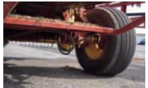
A hydraulic bale ramp is optional on the BR7070 and BR7090 for positive ejection of large 4' x 6' or 5' x 6' bales.
