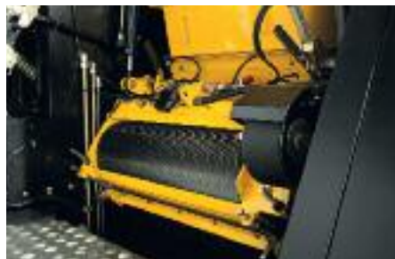
The optional kernel processor is in line with the cutterhead and measures a full 30 inches wide to spread crop over a wide area for precise kernel processing.
