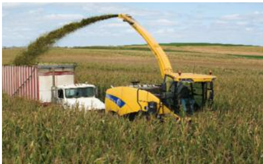
The 13-inch-wide FR9000 spout is a full three inches wider than previous FX models to handle increased crop volume. The 21-foot height allows you to easily fill trailers of any size.
