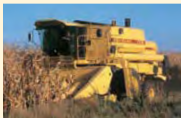
TX36 introduced to North American market with self-leveling shoe
