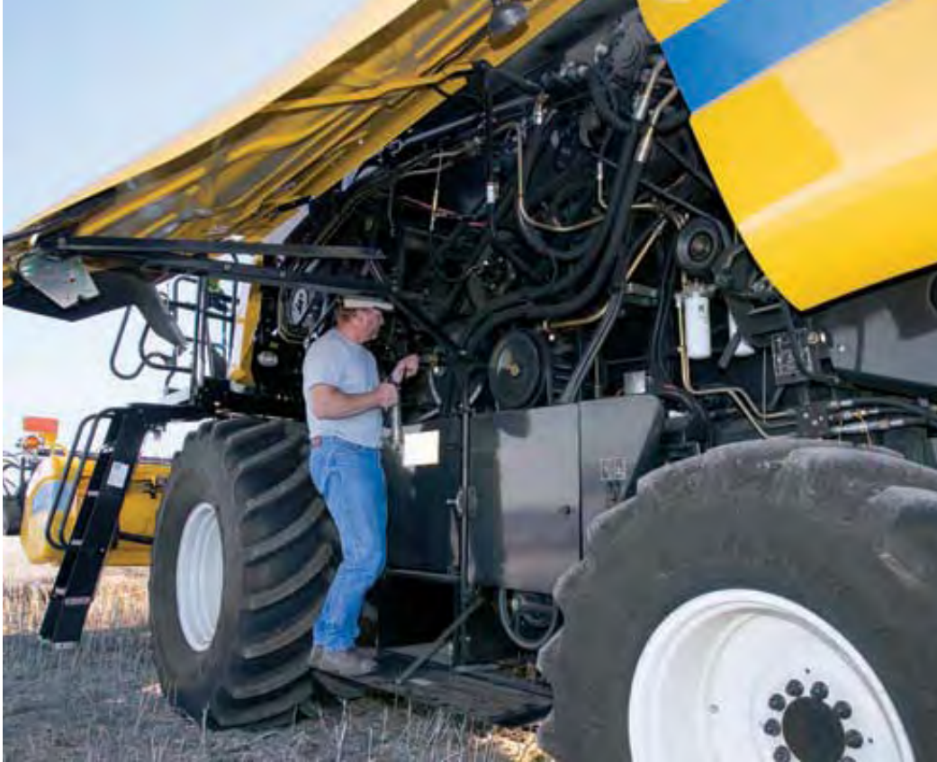
“Gull-wing” side shields provide complete service access.
