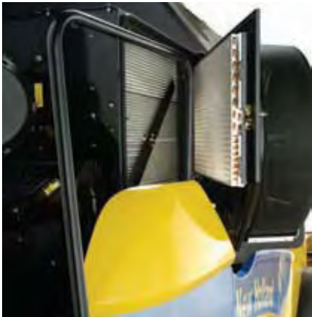
The CX8000 rotary air cleaner swings open for easy access to the radiator and hydraulic oil cooler
