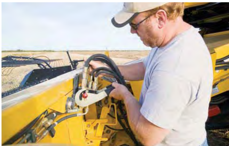
This hydraulic multi-coupler engages all hydraulic lines with one, over-center latch. It eliminates the need to hook up each header hydraulic circuit one at a time. It's a system that's quick, convenient and far less messy.
