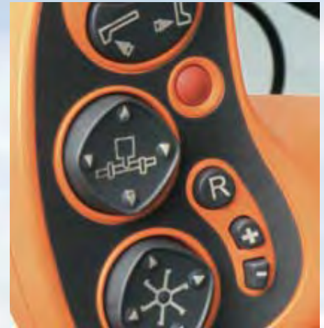
Terrain Tracer™ can be controlled manually with a switch on the hydrostatic lever.
