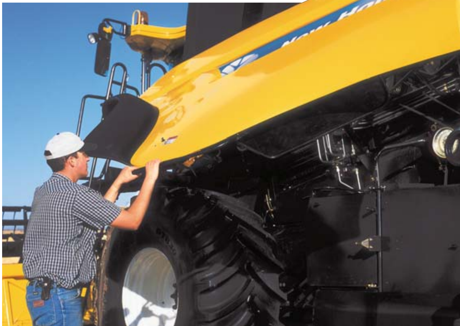
Rear service deck ladder folds down, making it easy to refuel or carry containers of fluid to the rear deck.
