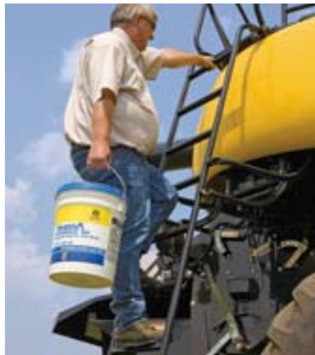
Rear service deck ladder folds down, making it easy to refuel or carry containers of fluid to the rear deck.
