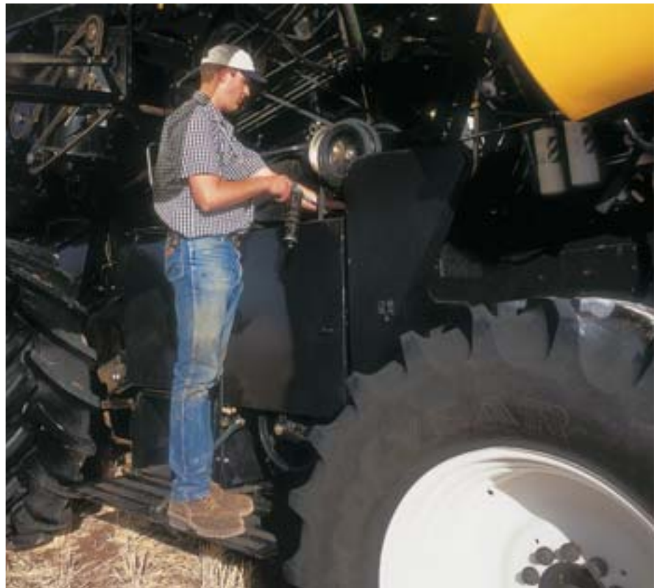
Service platforms provide secure footing and easy access.
