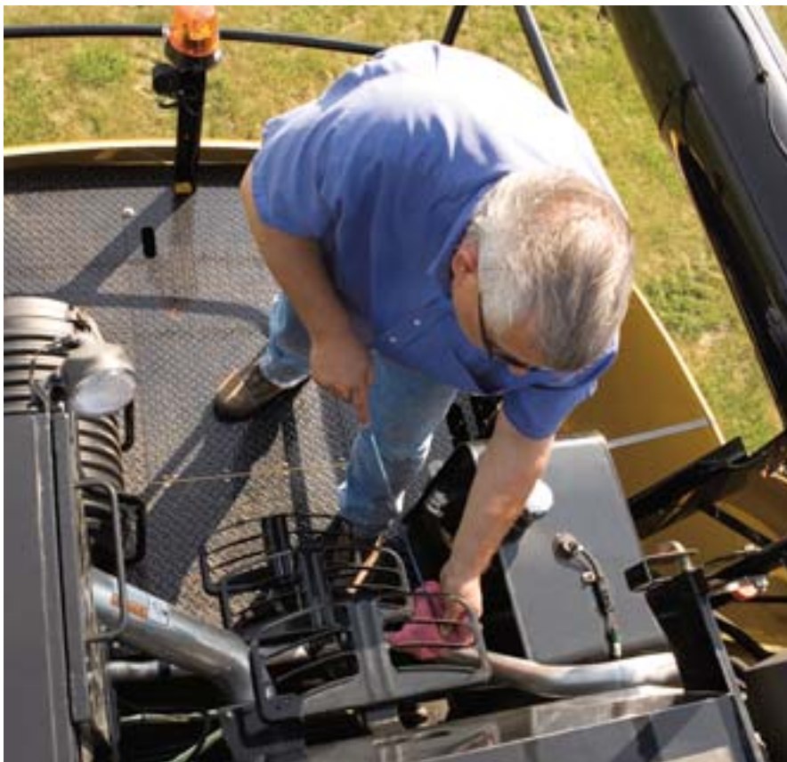
The rear service deck provides convenient access to the engine and grain tank.
