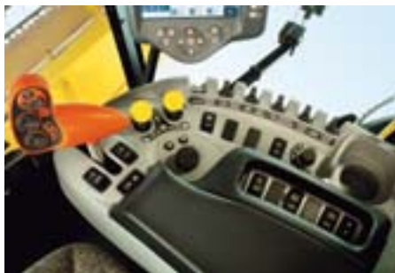
The right-hand armrest control console is the picture of efficiency, providing you with fingertip access to all cutting, feeding, threshing, separating and cleaning system controls using a natural motion of your arm.
