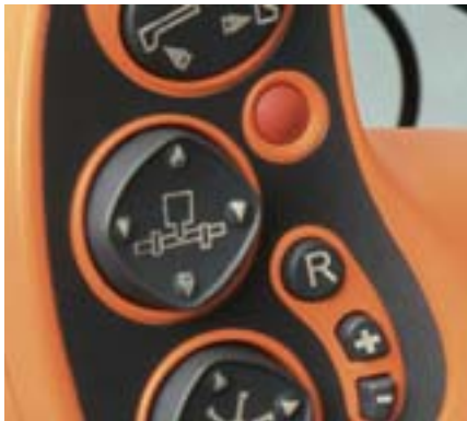
Terrain Tracer™ can be controlled manually with a switch on the hydrostatic lever.
