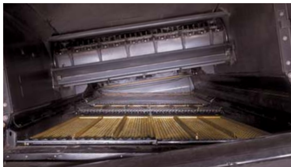
The SLS self-leveling cleaning system components (grain pan, cleaning fan and sieves) remain level while the lower main frame follows the ground contours. This allows grain to always remain level for maximum cleaning efficiency and setting forgiveness.
