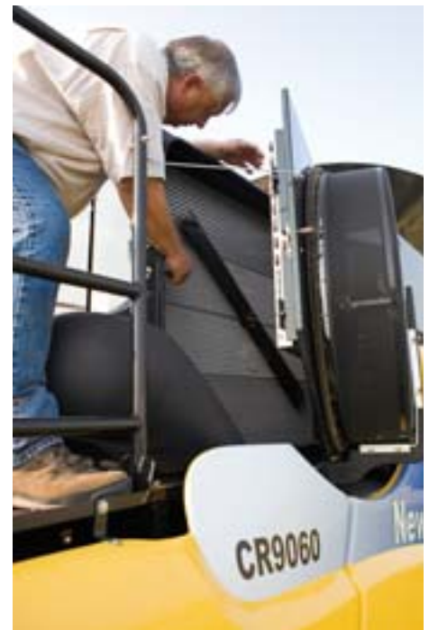
Accessing the rotary air screen, A/C condenser and hydraulic oil cooler is also a simple process from the rear service deck.
