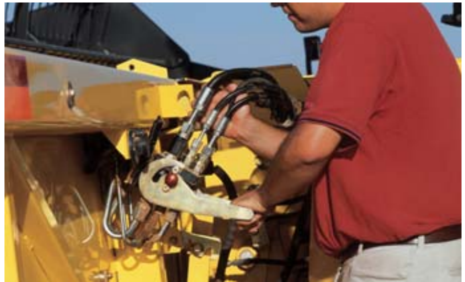
This hydraulic multi-coupler engages all hydraulic lines with one, over-center latch. It eliminates the need to hook up each header hydraulic circuit one at a time. It's a system that's quick, convenient and far less messy.
