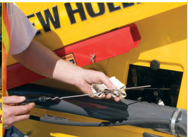
Access doors on side service panels open for fast daily maintenance checks.
