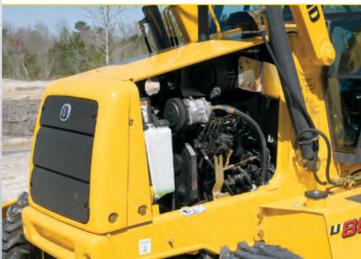
Side panels can be removed for complete engine access.
