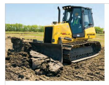
You can adjust PAT blade lift, angle, and tilt hydraulically to match the task at hand—finish grading, ditching, backfilling, or spreading.
