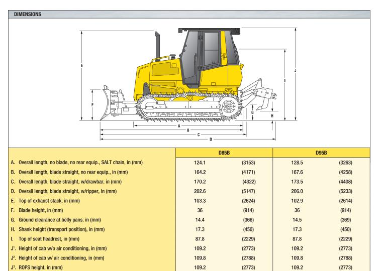
Note: Overall length is with blade pitch at 55° (factory setting). If blade pitch is adjusted to 60° length will decrease 15 mm (0.6 inches).
