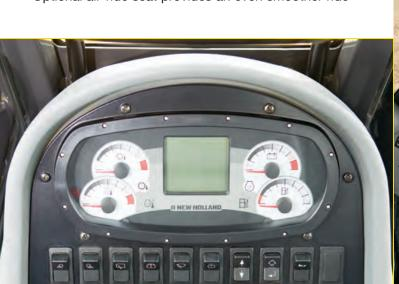
The instrument cluster provides system information with analog gauges and warning lights.
