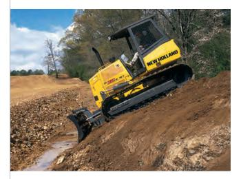
Wide-track machines are ideal for forestry operations, where ground conditions are relatively firm, but the machine regularly works on steep slopes.
