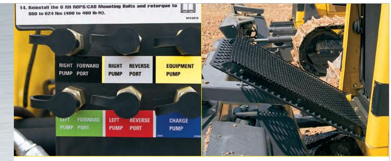
A centralized hydraulic diagnostic test panel easily verifies system pressures.
