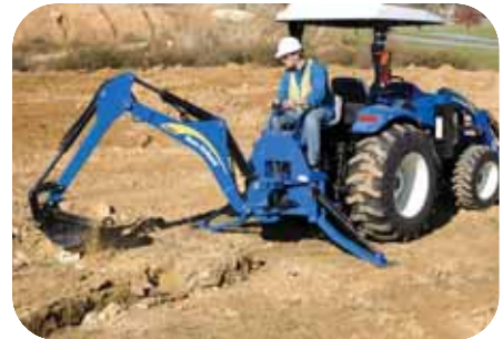
Utility backhoe allows you to work in tight quarters and dig to depths of 72 to 102 inches, depending on model.
