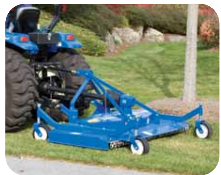
Rear-mount finishing mowers use an air tunnel design that provides smooth cutting even in tall grasses.
