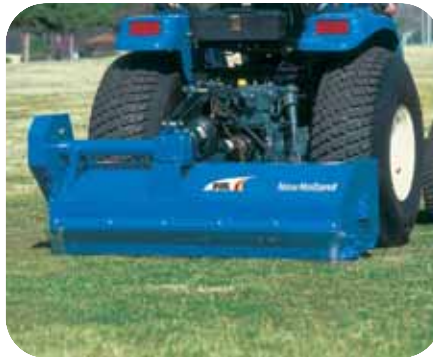
Flail mowers use fine-cut blades mounted to a horizontal rotor to shred clippings for a smoother more finished cut
