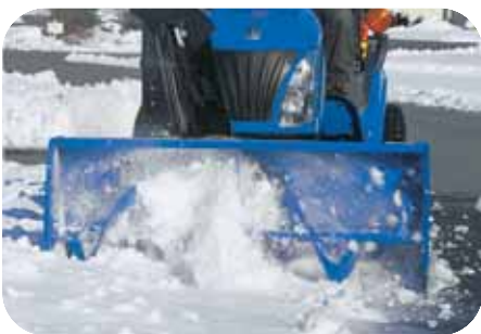
Front Quick-Attach snow blower cuts through snow up to 26 inches high, using a two-stage process to turn your Boomer into a powerful snow removal machine.
