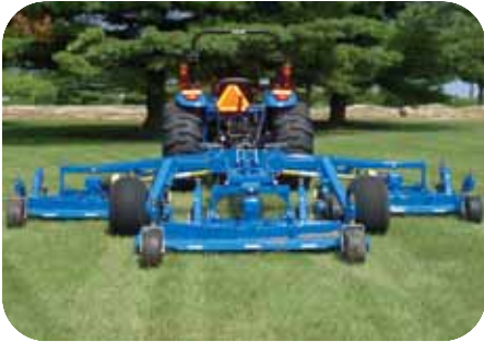
Flex-wing finishing mowers feature three floating mower decks that flex front-to-rear and side-to-side for precision mowing on the uneven terrain of golf courses, parks and other large areas.
