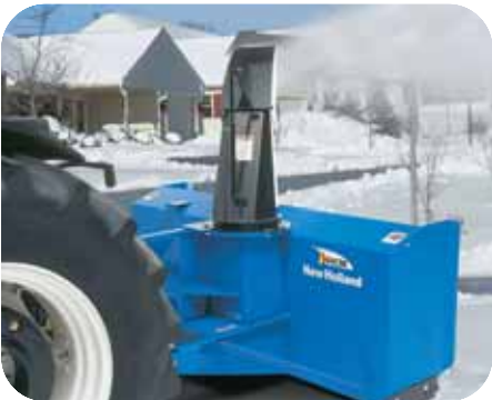
Rear-mounted snow blower uses a two-stage design to blow all types of snow—from light and fluffy to wet or hard-packed.
