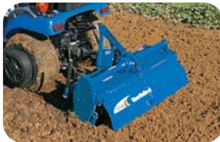
Rotary tiller uses curved steel tines to prepare seedbeds or control weeds between the rows.
