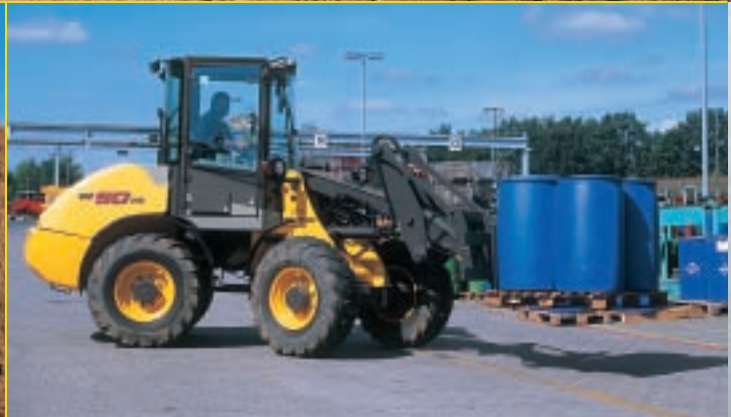
Precise, parallel forklift path eliminates the need for manual correction so operators can focus on load placement rather than load leveling.
