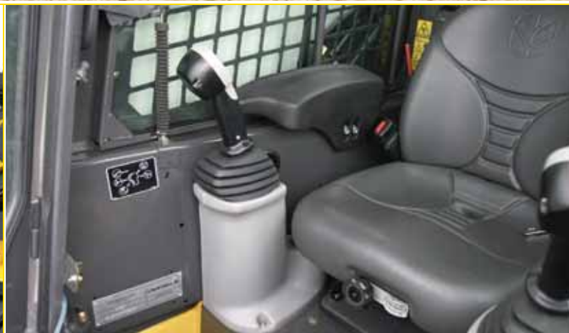
Adjustable armrests and suspension seat allow operators to find a comfortable working position.
