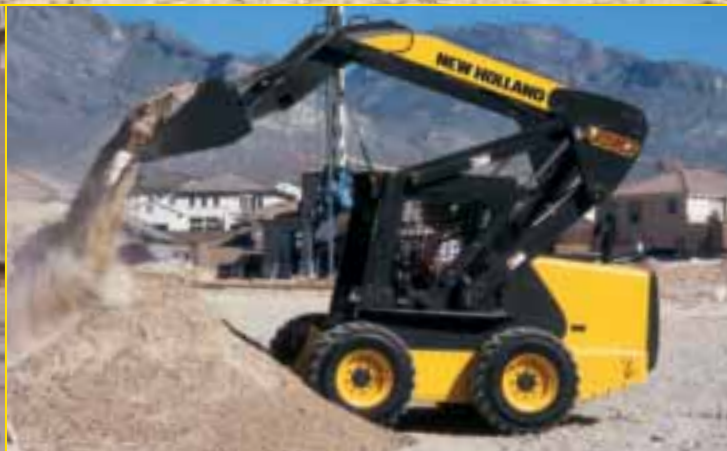
An exceptional 45° dump angle and 36° rollback angle help boost your productivity.
