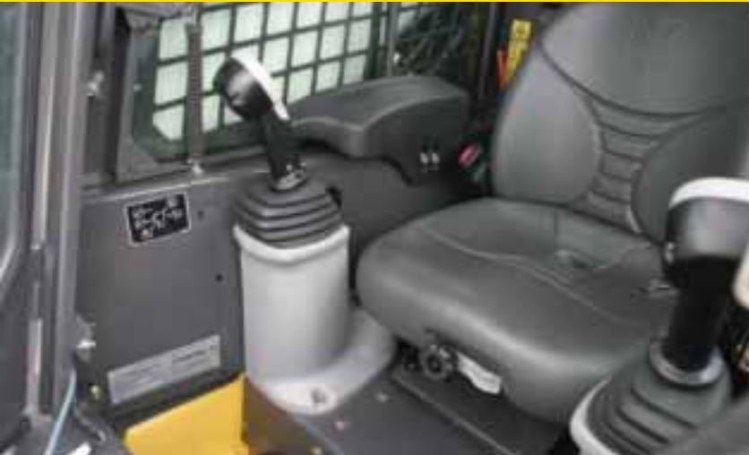
Adjustable armrests and suspension seat allow operators to find a comfortable working position.
