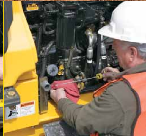
The swing-up hood allows easy access to site windows and fluid dipsticks and filters.
