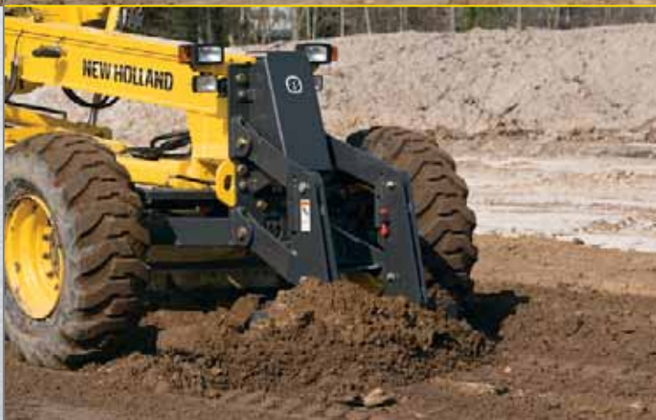
The front scarifier offers 20.75 inches of lift for excellent ground clearance and 12.5 inches of ground penetration.
