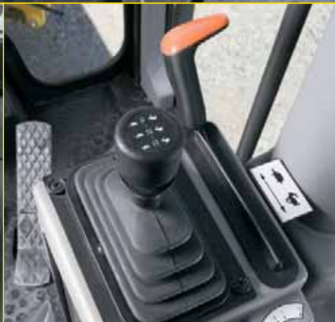
F-N-R bump shifter with eight forward speeds and four reverse speeds.
