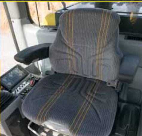
Adjustable suspension seat, arm rests and steering wheel allows each operator to achieve a comfortable position.
