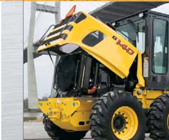
The fiberglass hood swings open assisted by charged cylinder supports. This provides easy access for routine engine maintenance.
