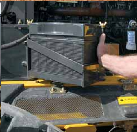
Two swing-out 1010 CCA maintenance-free batteries, one conveniently located on each side of the engine compartment.
