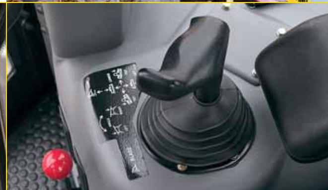
The palm-grip lever provides complete blade control.
