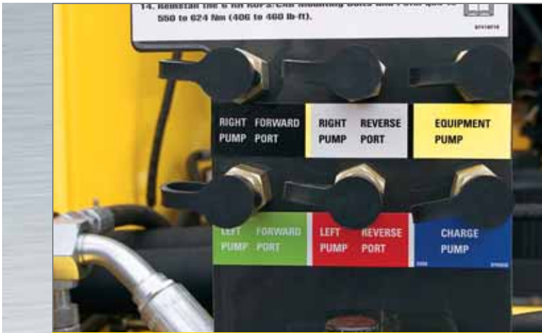
A centralized hydraulic diagnostic test panel easily verifies system pressures.
