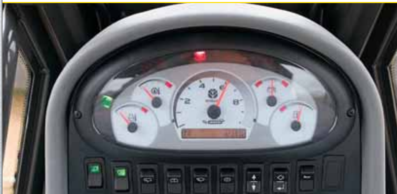
The instrument cluster provides system information with analog gauges and warning lights.
