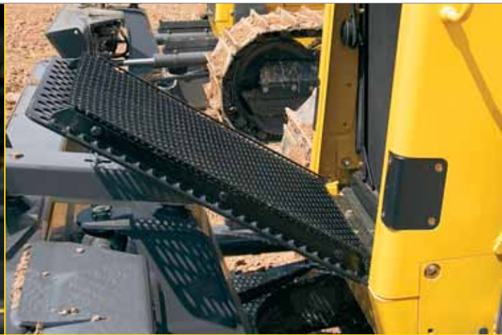
The hinged front grill allows easy radiator and cooler cleanout.
