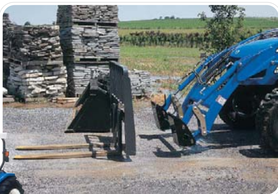
The optional Quick-Attach (skid steer loader compatible) faceplate increases attachment versatility and reduces the time to change between buckets and attachments.
