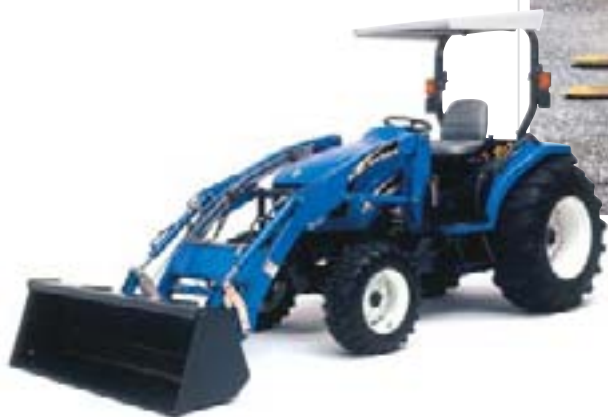
The optional Quick-Attach (skid steer loader compatible) faceplate increases attachment versatility and reduces the time to change between buckets and attachments.
