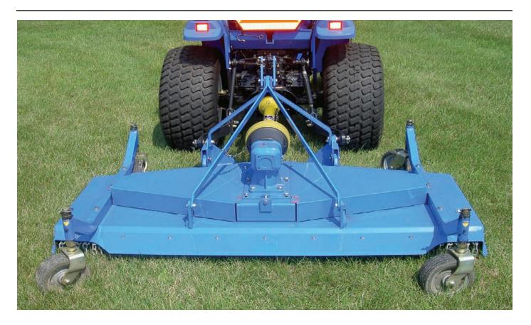
The 300 Series Rear Discharge Finishing Mowers are Category I, 3-point mounted implements for tractors equipped with 540 rpm PTO. These mowers are suitable for parks, golf courses, athletic fields, highway maintenance, farming, and homeowners.
