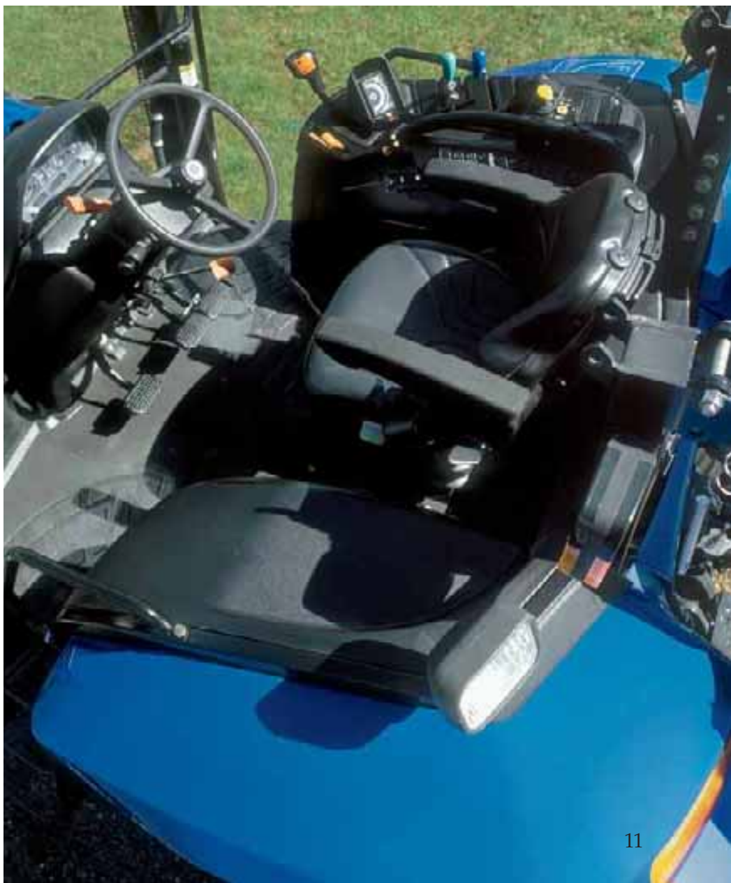
Controls for the three-point hitch and draft control are conveniently positioned for fingertip control. The loader control joystick, mounted on the seat, is designed to move with you for added comfort.
