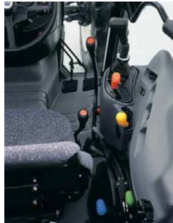
Speed and range levers are located within easy reach of your right hand.
