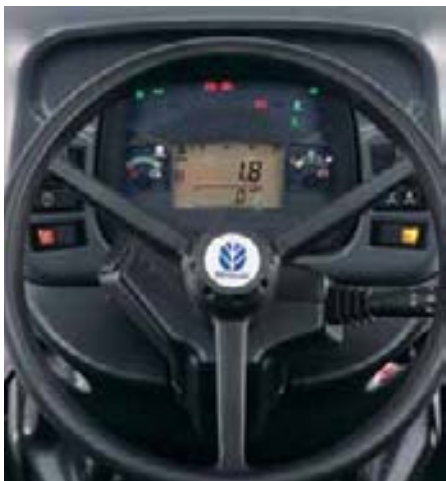
Digital readouts, analog gauges and a bank of indicator lights keep you informed with only a glance.
