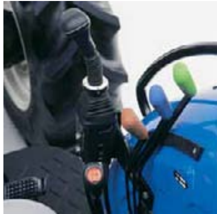
Controls for rear remotes and the loader joystick are conveniently located to your right.
