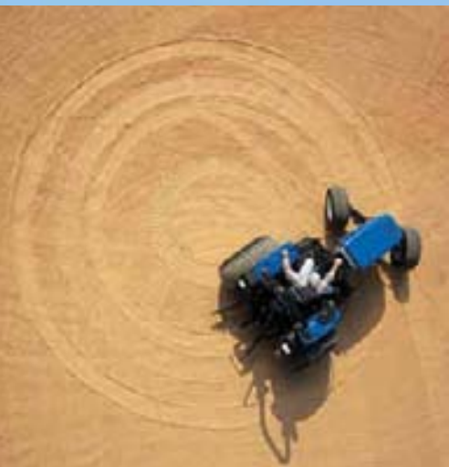
The SuperSteer™ FWD axle articulates as it turns, moving the outside wheel in front of the nose of the tractor and moving the inside wheel away from the tractor frame. This provides more tire clearance and a greater turn angle.
