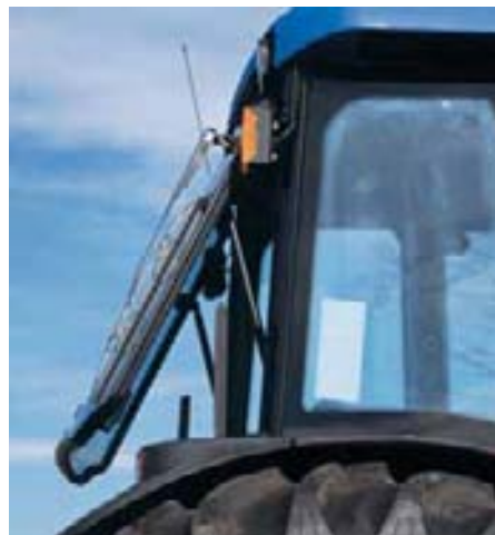
The rear window can be opened to three different positions. It opens fully, halfway, or can be opened only a few inches for ventilation.
