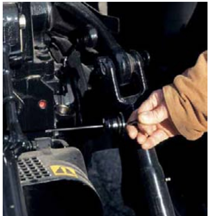
A single dipstick at the rear of the tractor allows you to check the oil level of the transmission, hydraulic and steering oil reservoir.
