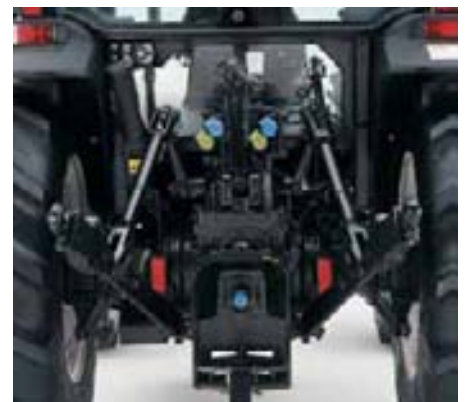
Remote valves are color-coded to match levers. Up to four rear remote valves are available.
