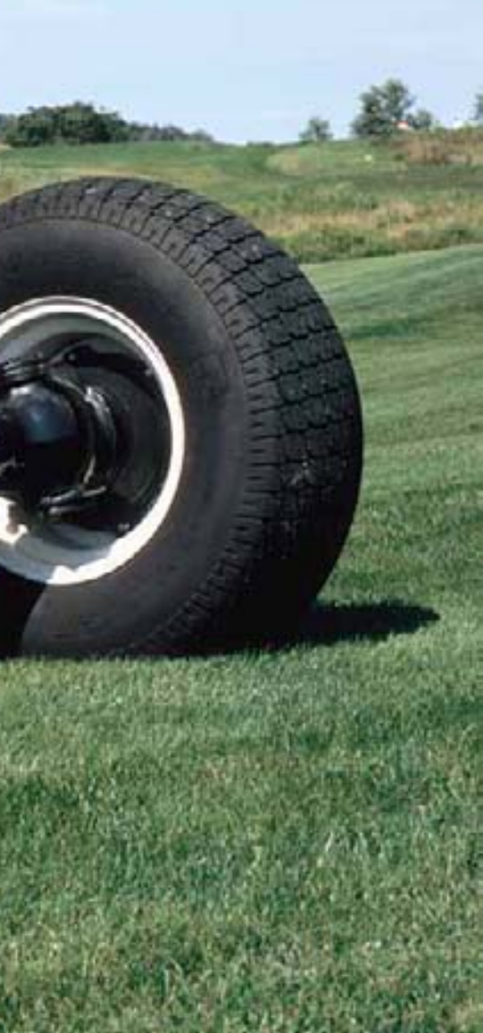
The SuperSteer™ FWD axle articulates as it turns, moving the outside wheel in front of the nose of the tractor and moving the inside wheel away from the tractor frame. This provides more tire clearance and a greater turn angle.
