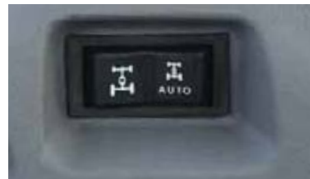
Operate the Traction Management System in the automatic mode, and FWD is engaged only when needed to save turf, tires and fuel.
