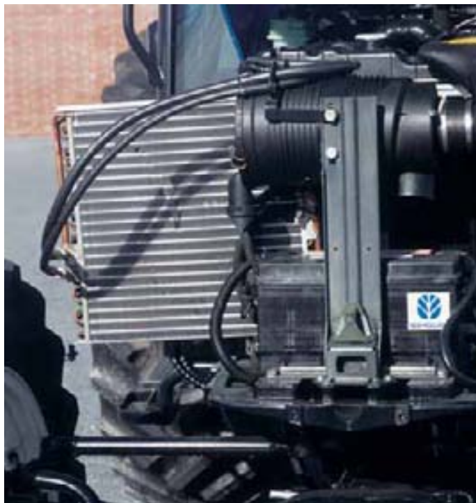
The hydraulic cooler slides out to the side for easy cleaning.
