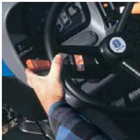
This power shuttle lever allows you to keep your hands on the wheel and shift from forward to reverse with your fingertips. It's the ideal choice for loader work.
