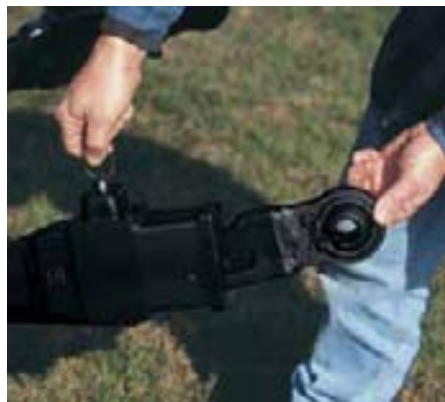
Heavy-duty, telescoping stabilizers and flexible link ends simplify implement hook-up.
