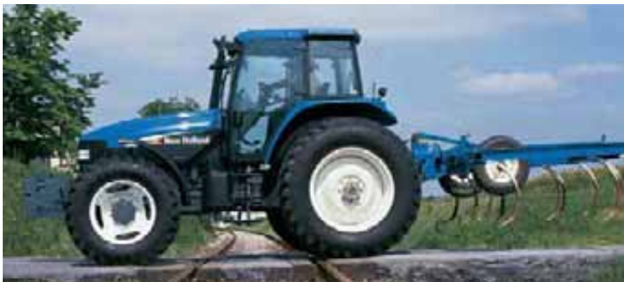
Dynamic Ride Control™ helps prevent three-point-mounted implements from “bouncing” on the rear hitch during transport. You enjoy greater steering control, added safety and a smooth, comfortable ride at speeds above 5 mph.
