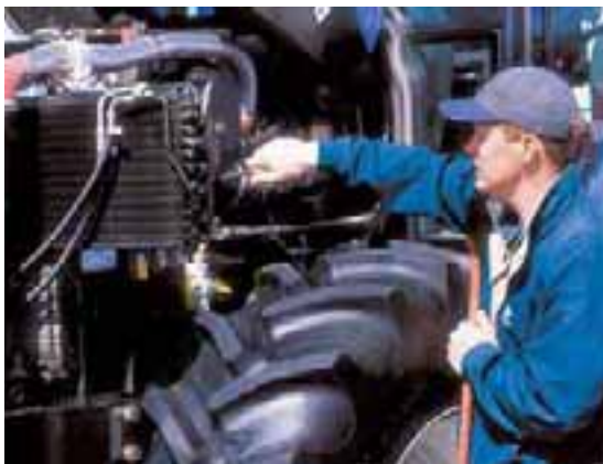
Clearing debris from the radiator is an easy job. The TM cooler and condenser slide out for inspection and cleaning, while most tractors require you to remove bolts, hoods and panels.
