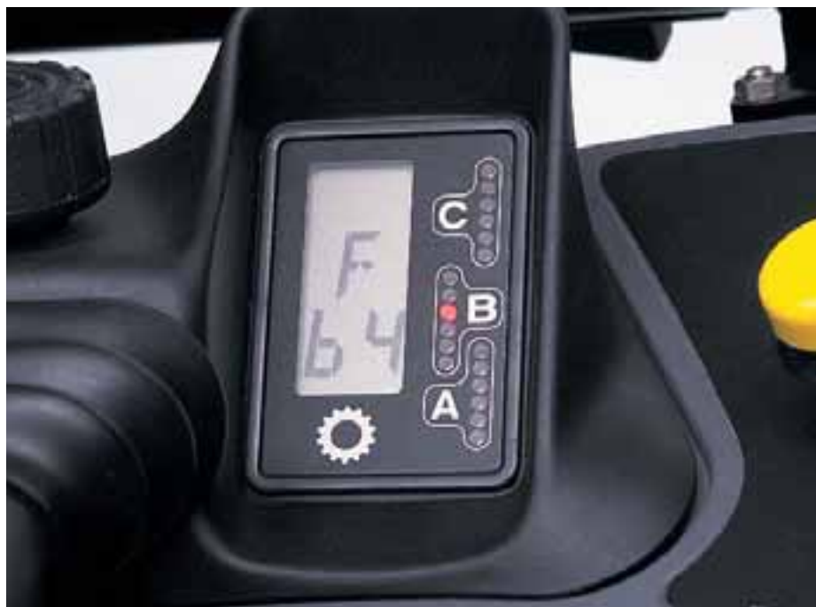
The Range Command™ display makes it easy to see which range and speed you're in. An audible beep and flashing LCD also remind you when a range change is required.
