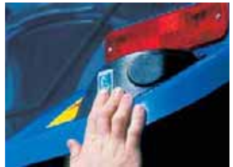
Rocker switches on the rear fenders allow you to raise and lower the three-point hitch for easy implement attachment and adjustment.
