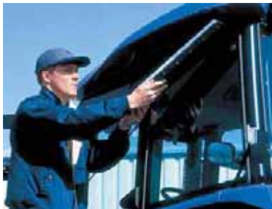
It's easy to reach the cab air filters right from the cab steps.
