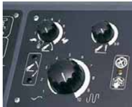
The Electrolink™ pod is located conveniently on the right-hand console for easy fingertip operation of the three-point linkage.
