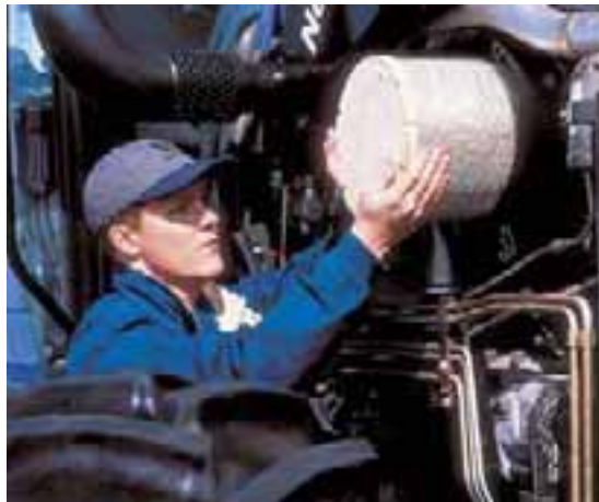
To access the TM air filter, simply raise the hood and remove a wingnut.
