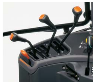
The new 20x16 mechanical transmission features a right-hand synchronized shuttle lever for easy forward/reverse shifts.
