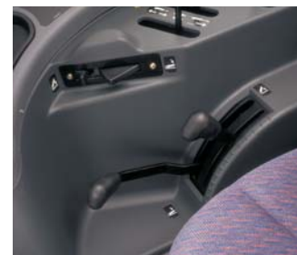
Mechanical hitch control features position, and draft control with the two levers located on the right side of the seat. You can raise or lower the implement with the push of a button.
