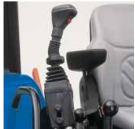
A convenient four-way joystick control is ideal for loader control.
