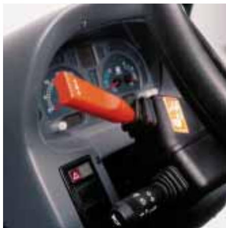
The power shuttle lever on tractors equipped with the Dual Command™ transmission allows you to shuttle from forward to reverse without clutching and without removing your hands from the wheel.
