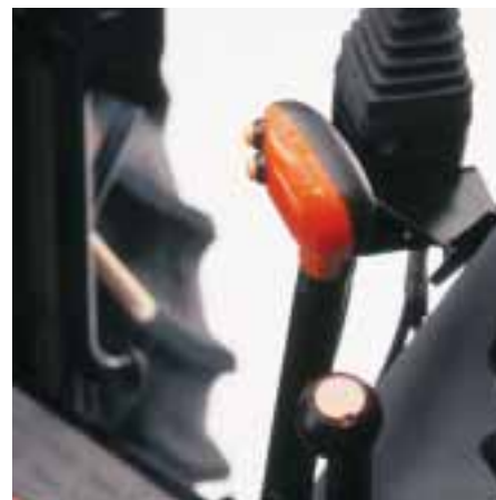
A push-button "powershift" in each gear doubles your speeds from 12 to 24 with the 24x24 Dual Command™ transmission.
