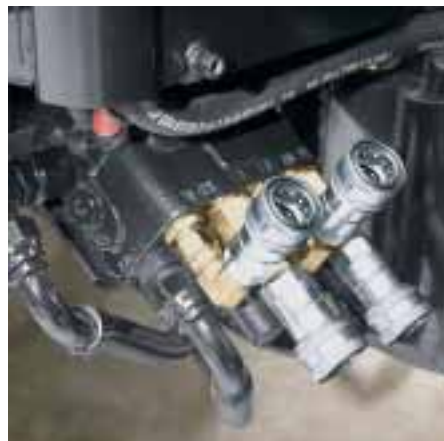
Mid-mount hydraulic valves make it easy to attach and remove New Holland loaders.
