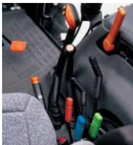
Speed and range levers for either transmission are located conveniently to your right and are easy to reach.
