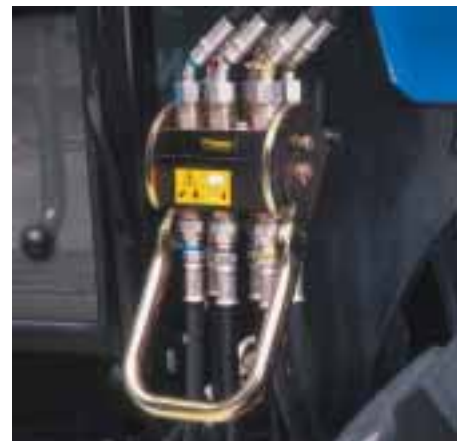
The optional Fast-Snap feature (52LC only) allows you to disconnect all four loader valves with one lever.
