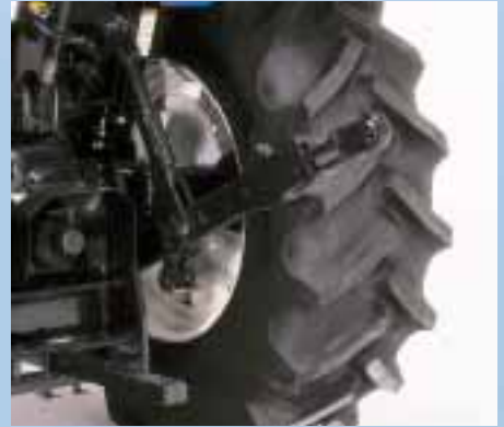
Telescoping stabilizers and flexible link ends make implement hook-up easy. (Flex ends are optional on Standard models).
