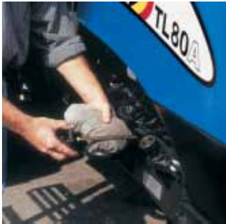
There's no need to raise the hood to check engine oil level.
