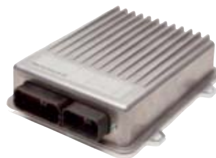
The Navigation Controller II receives user, satellite, correction and steering inputs and provides the control to guide the tractor. It includes three gyrometers and accelerometers for operation in uneven terrain.
