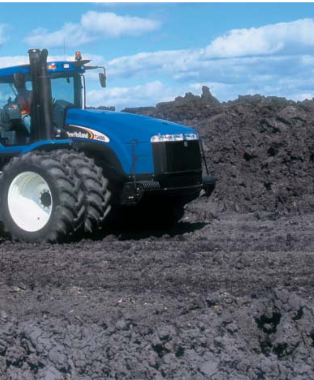
For scraping in large-scale commercial applications, the Precise Land Management Integrated Laser Leveling System allows the tractors electronics to automatically control depth on the 1st and 3rd remotes.
