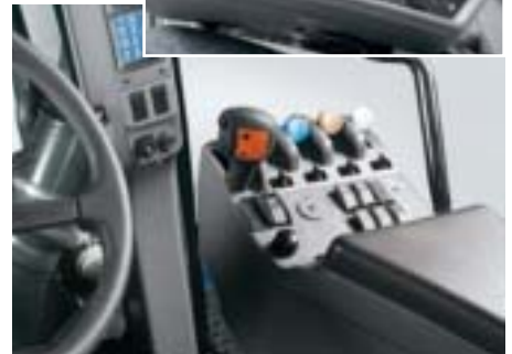
Right at hand ... controls for AutoShift™ hydraulic remotes, flow and timer, diff lock, hitch, custom headland management, optional slip limit, throttle and gear selection are integrated into the armrest for ready, comfortable access.
