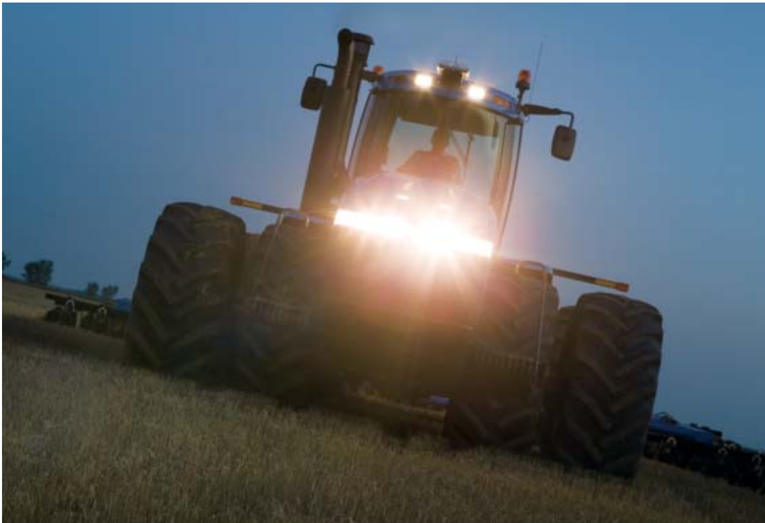
Up to 21 halogen work lights, plus optional High-Intensity Discharge (HID) lamps, brighten the night. You can adjust eight of the work lights to focus more illumination on areas in front of, behind and to the side of the tractor.
