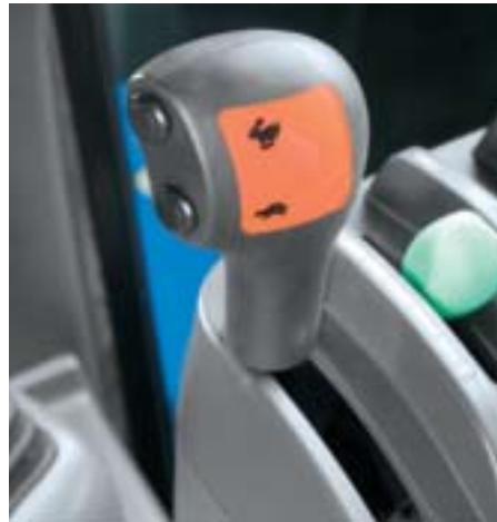
The Hi-Low shift on the 24x6 synchronized transmission is integral with the throttle lever for easy operation.
