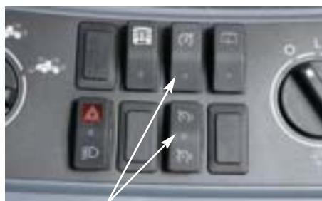
Use the constant speed switches to set the max RPMs and the speed adjustment switch or throttle to return engine speed to the desired level after making a turn.
