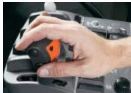
Change speeds with the touch of your thumb with the 16-speed powershift
