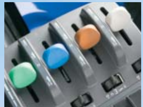
Hydraulic control levers and couplers are color-coded for ease of hook-up and to help track hydraulic operations.
