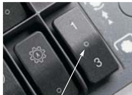
For scraping in large-scale commercial applications, the Precise Land Management Integrated Laser Leveling System allows the tractors electronics to automatically control depth on the 1st and 3rd remotes.
