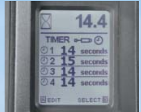
Performance instrumentation provides individual remote timers and a visual read out of flow control settings.
