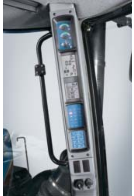
All the information you need on the go and at a glance — you can monitor everything from wheel slip and ground speed to fuel usage and hydraulic-flow readings with the optional performance instrumentation that's integrated into the cab post for easy viewing.
