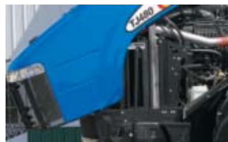
The cooling system provides the extra cooling capacity needed with higher-horsepower engines. The radiator is sized to the engine and can be accessed easily for cleaning.
