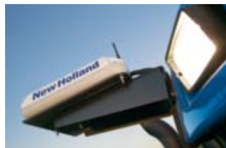
The New Holland 252 antenna receives the GPS signals to guide the vehicle. This antenna can easily be transferred from tractor to tractor or even to your combine.
