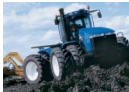
TJ engines produce from 380 to 530 hp and also give you up to 40% torque rise and power growth of up to 54 hp. That's more than enough power and torque to pull the heaviest carry-all scraper in the harshest conditions.
