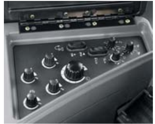
You have fingertip electronic control of the three-point linkage and draft settings.
