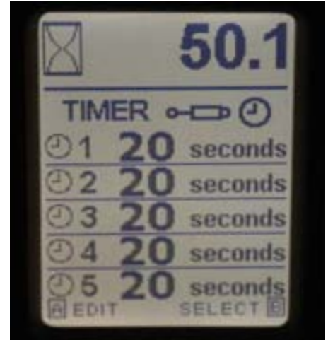
The optional Performance Instrumentation monitor gives you full control of the timing and flow of each valve independently and provides an on-screen report of flow rate and timing.
