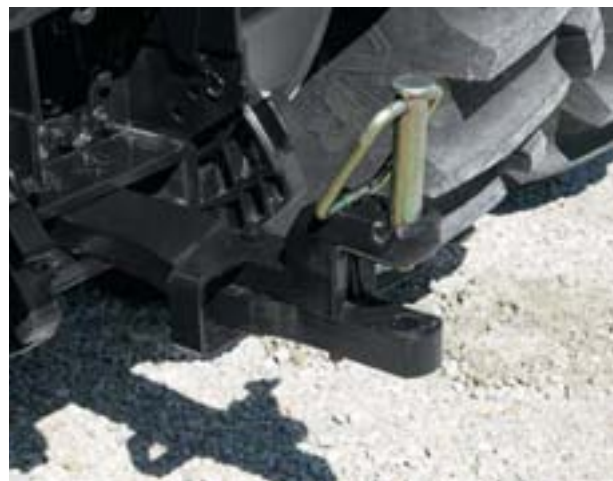
Hydraulic top link option for ease of implement hook up and in field adjustment.
