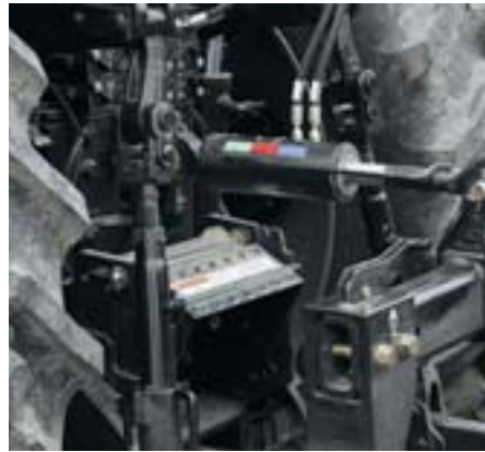
Hydraulic top link option for ease of implement hook up and in field adjustment.
