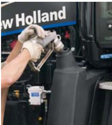
The fuel tank fill point is right beside the steps where it can be filled easily from ground level.
