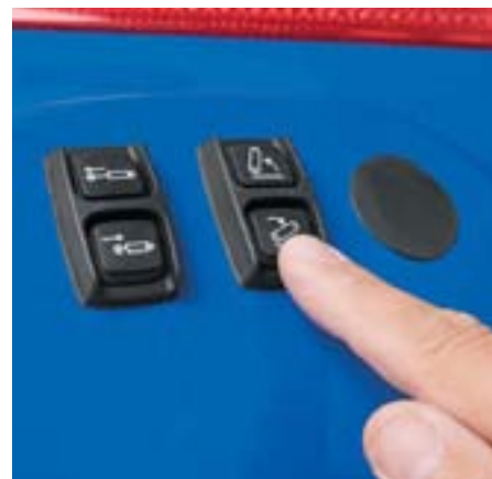
Remote three-point hitch and hydraulic Top Link rocker switches are located on the fenders for added convenience.
