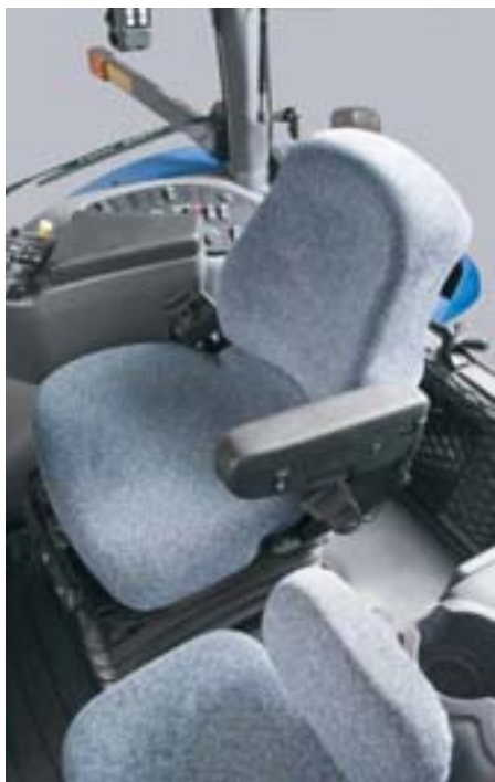
The standard air suspension seat provides deluxe comfort. An instructor seat can be installed in place of the workstation area to your left.
