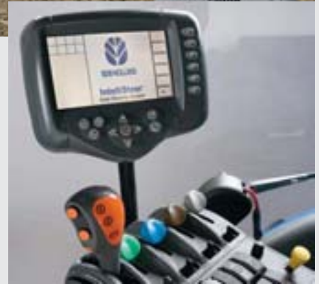
Use the IntelliView™ II color monitor mounted on the right-hand armrest to control the IntelliSteer™ auto steering system.
