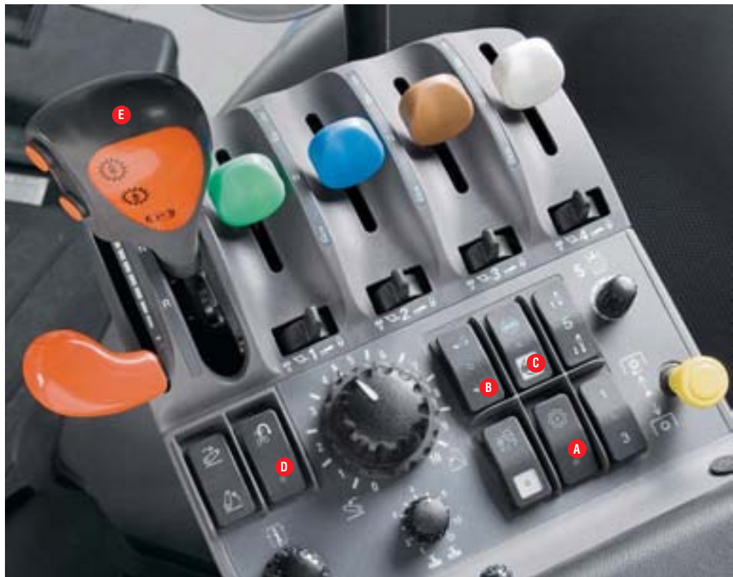
Switches are conveniently located on the right-hand armrest control console for A) AutoShift, B) front-wheel drive engagement, C) Automatic Diff Lock, D) Custom Headland Management, and E) transmission control lever.
