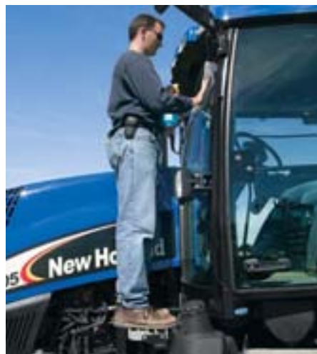
An optional front window step allows for easy window cleaning and provides access to the top of the cab, front wiper, and front cab roof lights.
