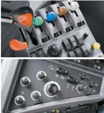
Color-coded hydraulic remote levers allow you to easily keep track of hydraulic operations. Remote valve flow controls, master timer and secondary three-point hitch controls are located under the armrest.
