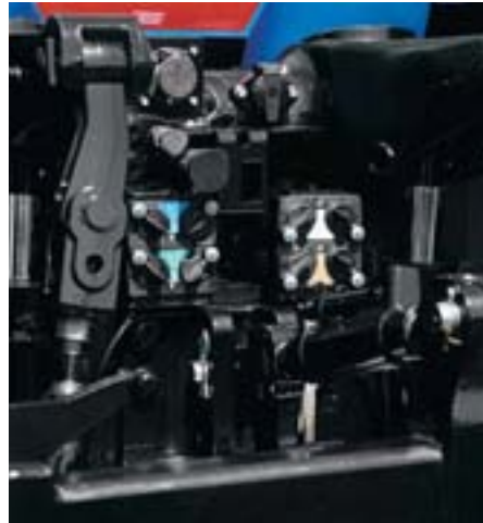
Quick couplers allow for easy coupling under pressure and are color-coded to match the in-cab remote levers.
