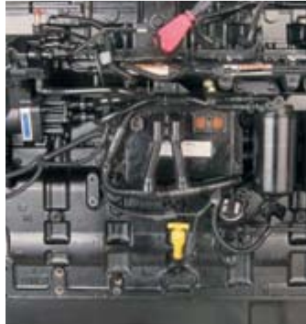
A new common rail fuel injection system boosts TG Series II tractor fuel efficiency. An electronically controlled injector supplies precise quantities of high pressure fuel from a common rail accumulator to each individual cylinder, eliminating plunger pumping elements and long individual injection lines to each cylinder.
