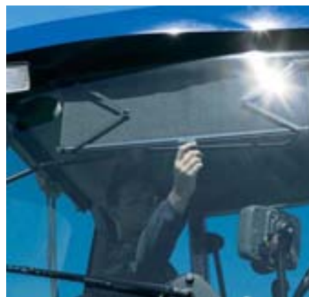
Add the windshield wiper and sunscreen options for the right-hand window for clear views no matter what the weather. Wiper/washers for the front and back, and a front sunscreen are standard.
