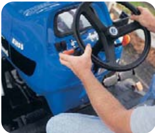
Shuttling between forward and reverse is as easy as moving the shuttle lever which is located to the left of the steering wheel.
