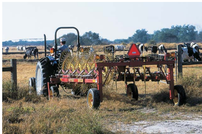
The HT152 standard and HT154 deluxe wheel rakes both fold down to a narrow 8' 3" for easy transport. The hydraulic-fold frame lets you change between transport and field positions right from your tractor seat.
