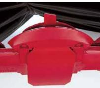
Skid shoes are 1/4" thick and 8" wide to protect the disc modules from obstacles. They extend behind the module several inches for optimum flotation and extended wear life of the shoe. Their unique shape works with cutterbar tilt to provide a broad range of cutting heights.
