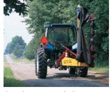
**Cutterbar transport lock** engages automatically for a secure hold. Just pull the cord to release.
