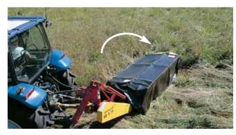
A spring-loaded breakaway latch protects the cutterbar by allowing it to swing back the instant an object blocks the cutter path. Simply back up to re-engage the latch.
