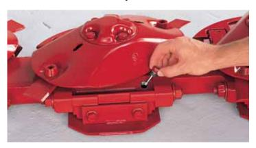
Cutter bar service couldn't get much easier. Check the oil in the modules every 50 hours with the convenient dipstick provided in the cap. Change the oil once a seasen or every 200 hours. For even more convenience, only one type of oil (80W90,GL5) is needed for all locations.
