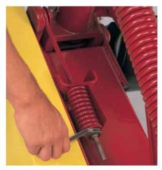
Exclusive V-belt tension spring has an easy-to-see tension indicator so you can check belt tension at a glance. Adjusting tension is easy, too — there are no shields to remove. All it takes is the turn of a nut.
