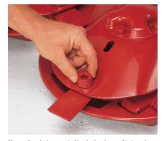
**Heavy-duty knives** are double-edged and reversible for twice the mowing life. Changing them is a snap — you don't have to bother raising the cutterbar like some competitors. Bolts are located on top for easy removal with the disc in any position.
