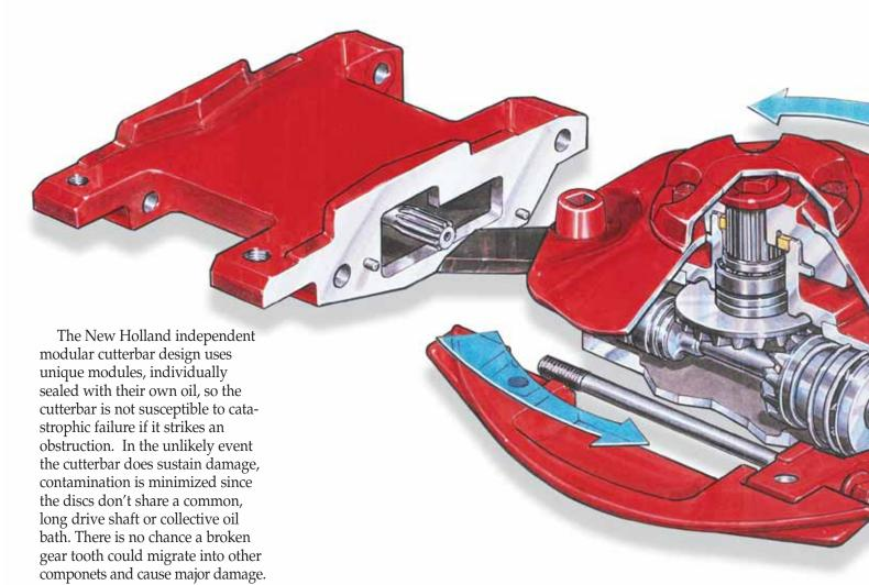
Each module is driven by short, independent, heat-treated and splined drive shaft sections that reduce replacement cost and make repair easy. Simply remove the tie bolts, and in minutes you can slide a module or spacer off for repair or replacement.
