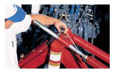
**Convenient jack stand storage and installation.** Remove the tethered pin to install the jack. Flotation spring force is released automatically
