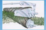
crimp and crack stems evenly along the entire length of the plant, so you get fast drydown yet retain protein-rich leaves. Adjusting roll pressure is easy. No tools are required. Critical roll gap adjustment is made with one adjusting bolt per side, no removing or adding shims.
