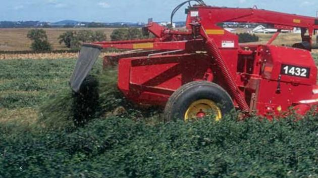
tive flails — allowing the cut crop to lay on top of the stubble for better air circulation and more thorough drying.
