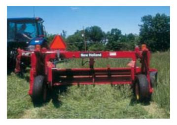
tongue design you can enjoy swivel hitch-like convenience and performance without the need for a three-point hitch or drawbar extension. You can mow at most any angle and make square and over-square corners without vibration or noise.
