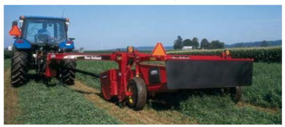
Adjustable header flotation springs and on-the-go cutting angle adjustment allow you to get all the crop without scalping or knife damage.
