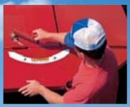
A simple turn of a hand crank lets you raise the conditioning hood away from the flails for lighter conditioning. Lower the hood for more aggressive action in grass. (Model 1412 shown)
