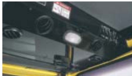
Adjust the direction and flow from the overhead air conditioning and heater vents for maximum comfort.
