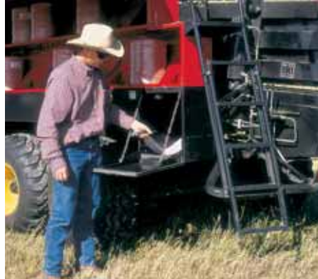
Two large storage containers—one on each side of the baler—are sealed from dust and can be locked, providing convenient storage for twine and tools.
