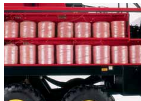
Large twine boxes allow both the BB940A and BB960A to carry 30 balls of twine — plenty for a full day of baling
