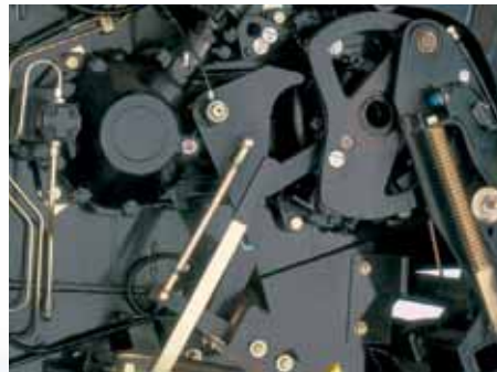
The self-contained hydraulic system is electronically controlled, supplying oil to two hydraulic cylinders at the back of the baler that apply pressure to three moveable rails on the top and both sides of the bale case.
