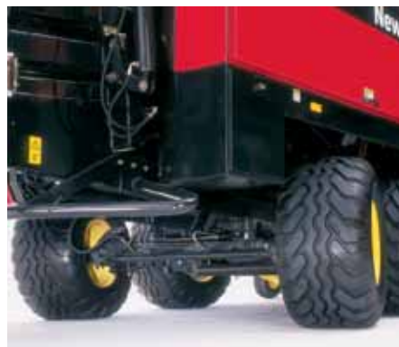
Auto-Steer™ tandem axle allows you to lock the rear wheels for transport and unlock them from the tractor cab to make sharper turns without tire scuffing and field damage.
