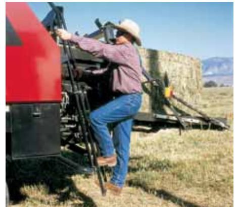
A knotted access ladder provides a convenient route for servicing (optional Rotor Cutter shown).
