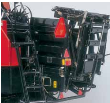
Gas struts assist with the folding of the bale chute. The roller bale chute (shown) folds hydraulically and is automatically secured for transport
