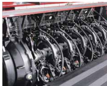
Four knotters on the BB940A and six on the BB960A are driven by a fully enclosed gearbox to ensure positive tying and a long working life.
