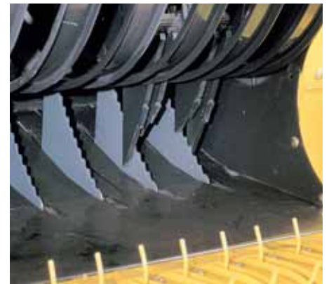
Rotor cutter knives are held in this knife drawer. It conveniently slides out for simple knife inspection, sharpening or changing.
