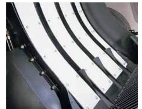
The fill-flow floor — a CropCutter™ baler exclusive — features plastic floor extension strips to reduce friction and grooves for the stuffer fingers to follow, resulting in smoother feeding in high-moisture conditions, better top filling and reduced load on the stuffer fingers.
