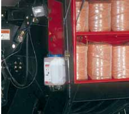
The automatic chain oiling system uses this large, five-liter reservoir to reduce fill-ups.
