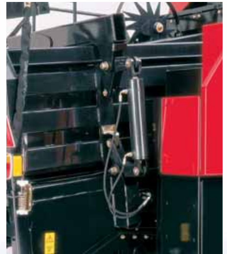
The self-contained hydraulic system is electronically controlled, supplying oil to two hydraulic cylinders at the back of the baler that apply pressure to three moveable rails on the top and both sides of the bale case.
