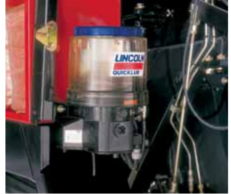
A standard, automatic greasing system supplies grease from this master dispenser to the five grease blocks.
