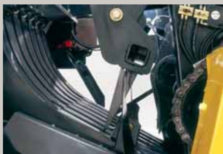
Crop from the feeder is pushed into the crescent-shaped precompression chamber where the material is compressed into a "slice" of preset density.
