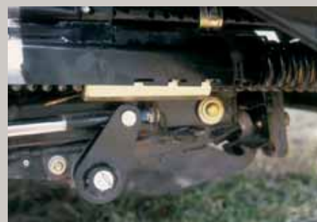
Adjusting the pickup is easier than ever. Sliding collars and retaining pins allow you to change flotation and height without tools or limiting chains. And, you can adjust windguard height with one chain located on the left-hand side.
