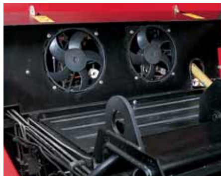
A constant flow of air from knotter fans — two on the BB940A and three on the BB960A — keeps the tying area clear of dust, chaff and twine tails to help prevent mis-ties. You control them through the InfoView® monitor
