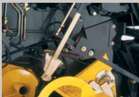
This spring-loaded handle allows you to adjust (without tools) bale shape and density by changing the amount of hay compressed into each slice delivered into the bale chamber. This is a time-saver when changing crops.
