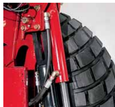
“Stop” cylinders on each lift arm make it easy to return to the pre-set cutting height after each pass.
