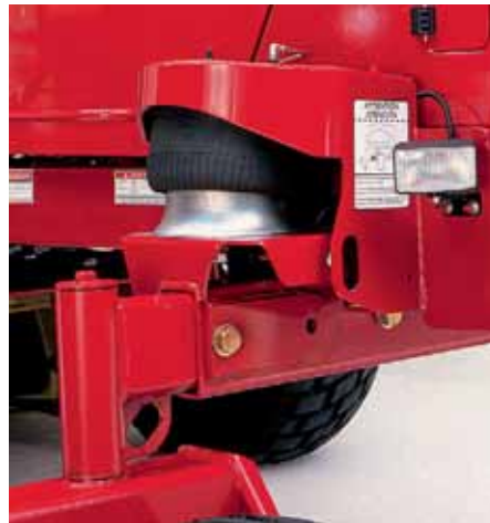
The new independent rear axle suspension reduces operator fatigue and stress on the machine.
