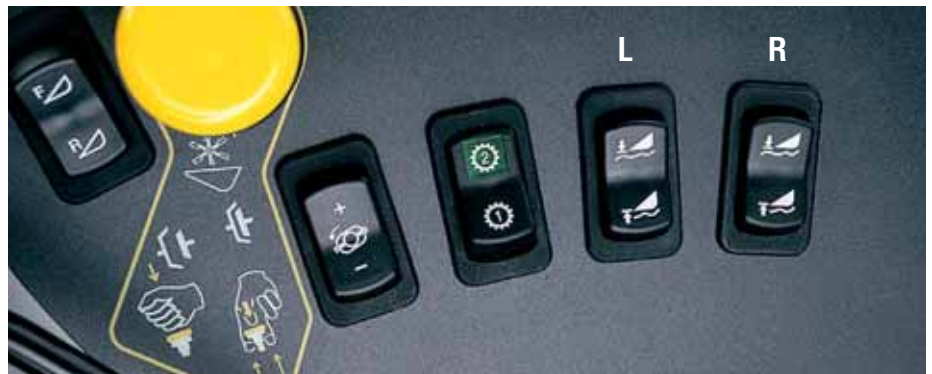
Dual switches in the HW345 and HW365 cab allow you to control the flotation of the left and right side of the header independently.
