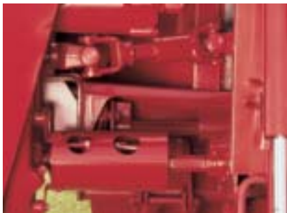
Dependable gearbox drives the conditioning rolls. No chains to adjust!
