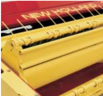
5-bat reel provides more uniform crop flow.
