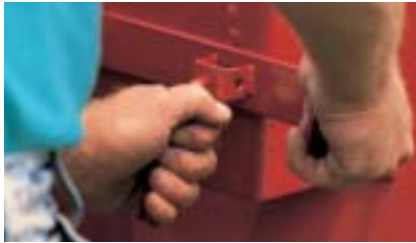
Swath to windrow – No tools needed and the change takes only seconds.
