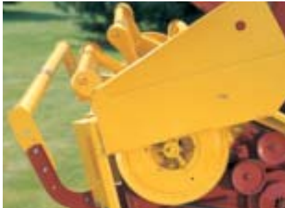
Hinged shielding provides easy access to knife and reel drives.
