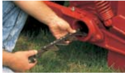
Spare knife assembly storage space is provided in the pipe frame of the machine.
