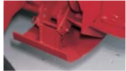
Adjustable header skid shoes allow quick and easy cutting height adjustment.
