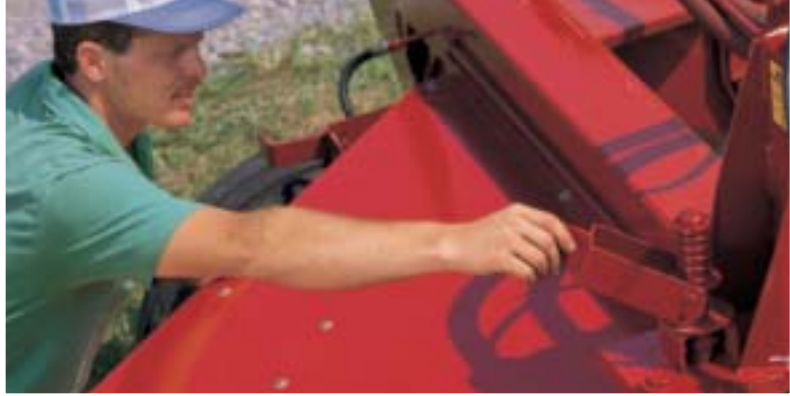
The spring-loaded tongue lock is easy to latch, so you don't waste time when you're ready to transport.
